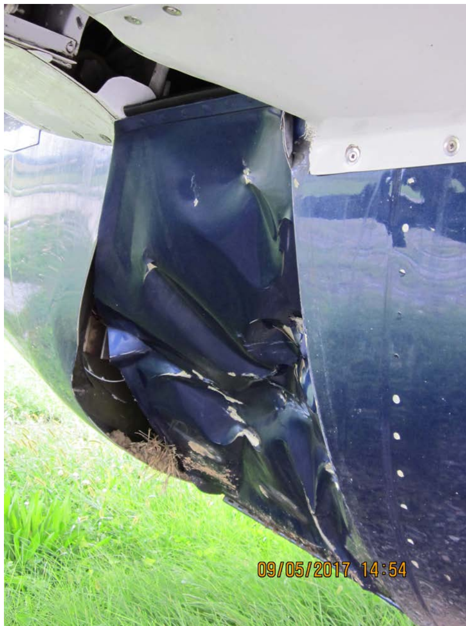
Photo 3 – View of fuselage buckling under right wing (courtesy of FAA)
