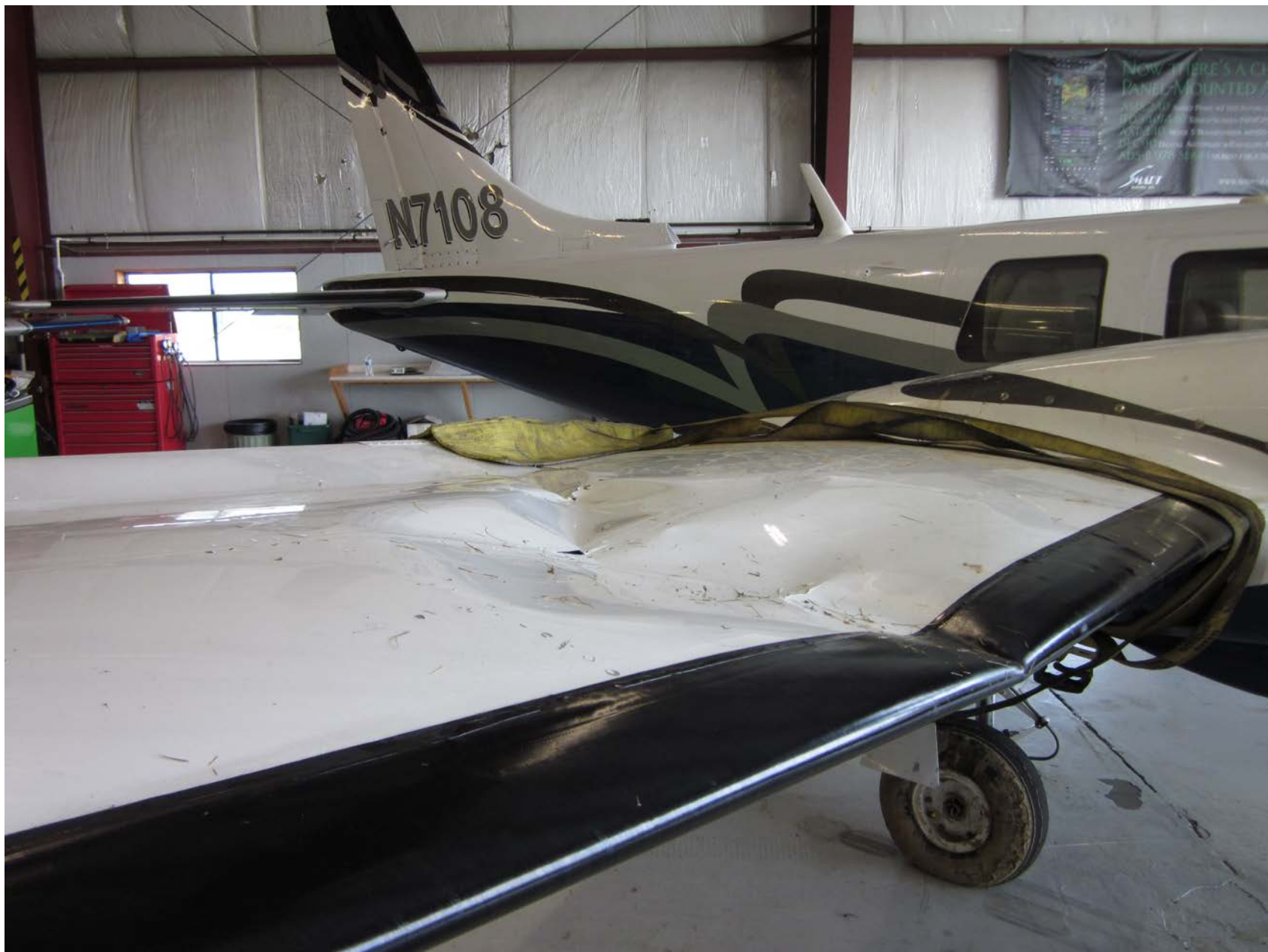
Photo 1 – Forward view of right wing buckled outboard engine nacelle (courtesy FAA)
