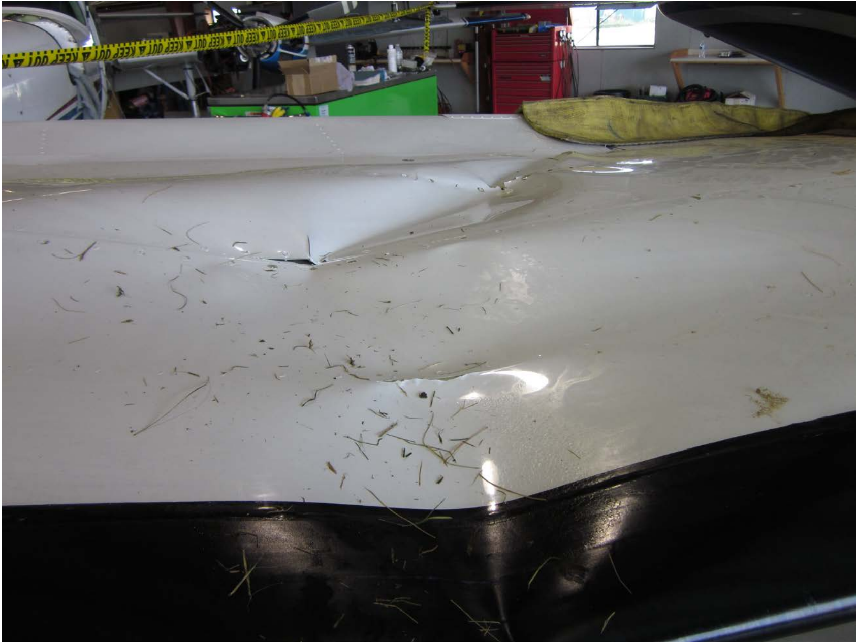
Photo 2 – Close up forward view of buckled right wing (courtesy of FAA)
