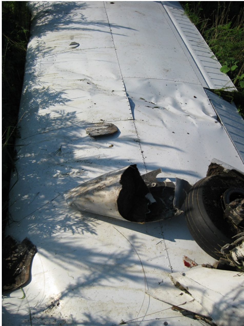
Photo 2 – FAA Digital Photograph. View Depicting the Damage to the Left Wing
