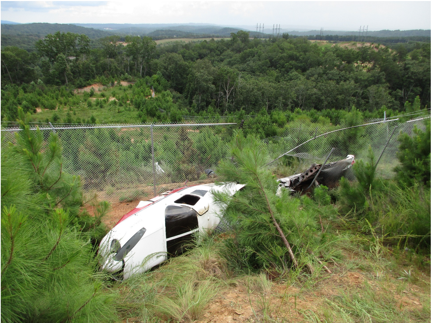
Photo 3– View of fuselage off the end of runway with wings separated (courtesy of FAA)
