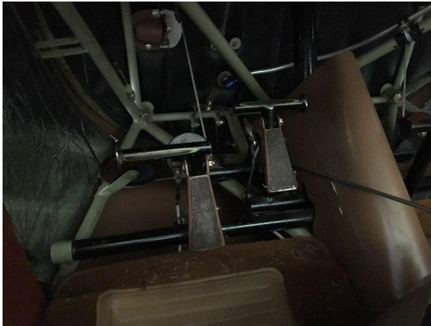
Heel brake pedals installed at left cockpit seat position
