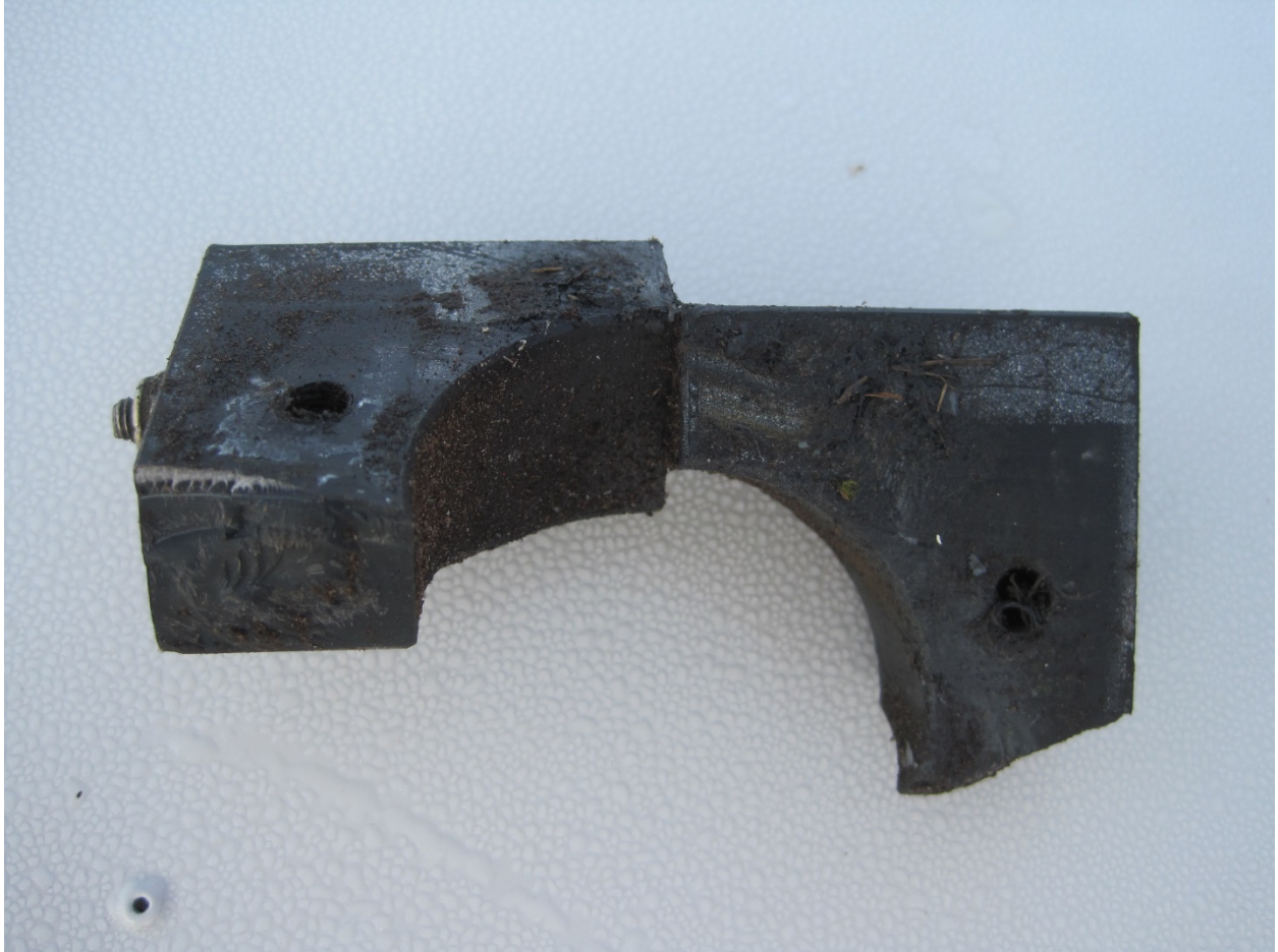
Figure 3 Fractured lower nose gear bearing (Photo courtesy of the FAA)
