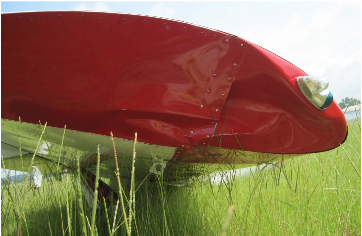
Figure 2 Damage to the right wing (Phot courtesy of the FAA)
