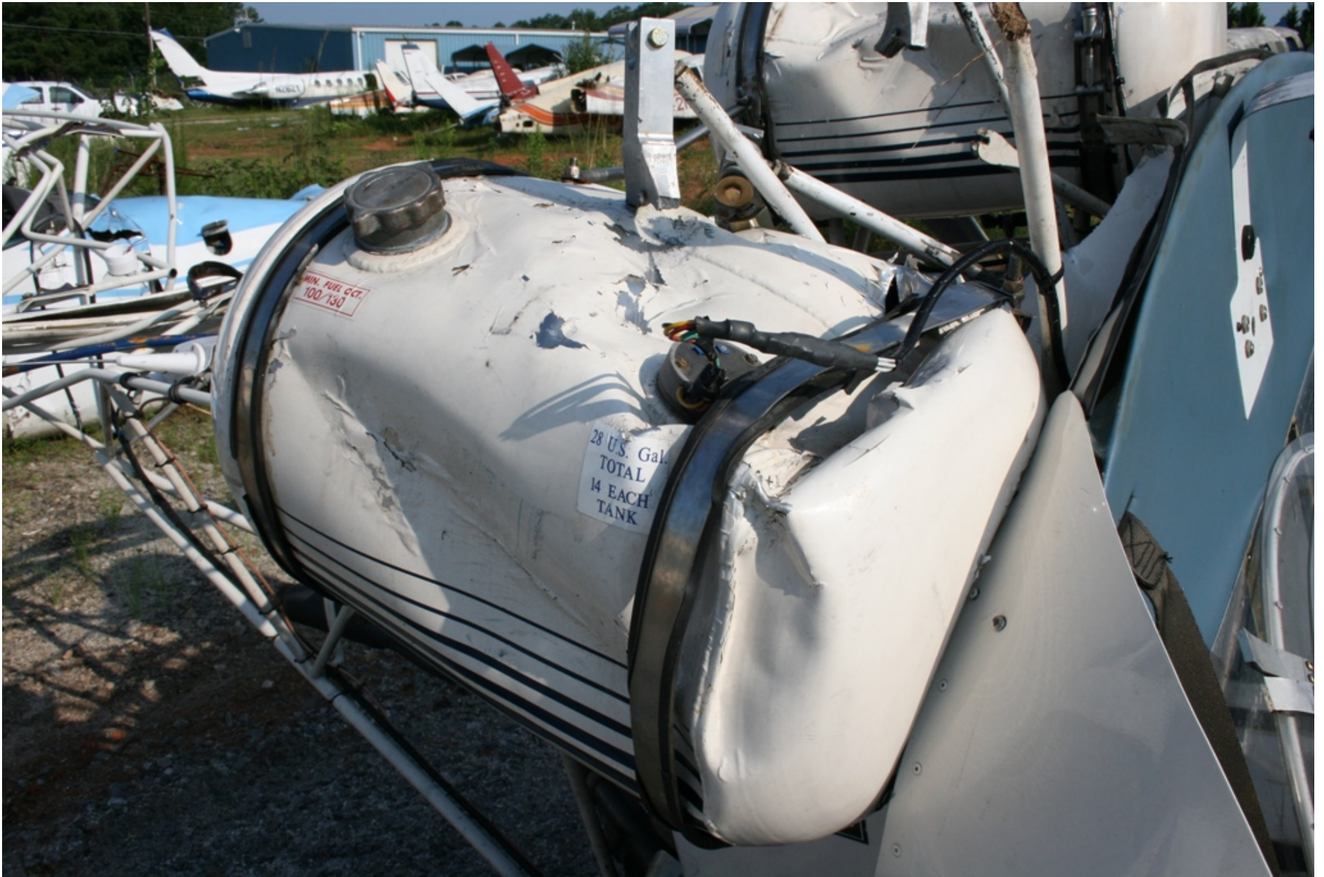
Photo 5 – Fuel Tank Damage (NTSB Photo)
