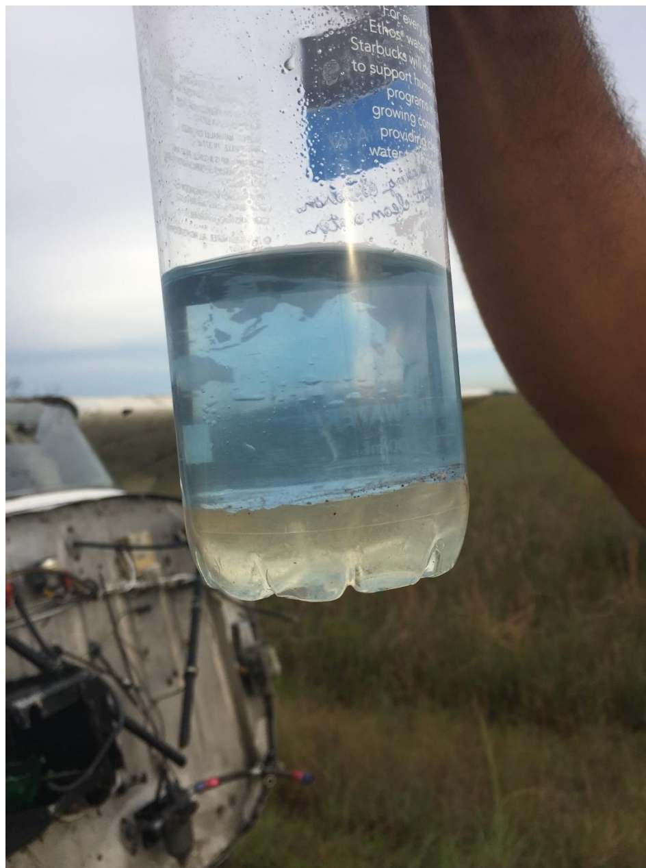
Photo 2 – Water in fuel sample (FAA)
