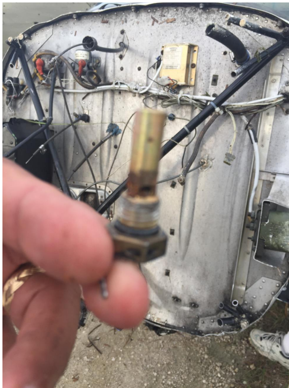
Photo 3 – Fuel drain sump valve, rusted (FAA)
