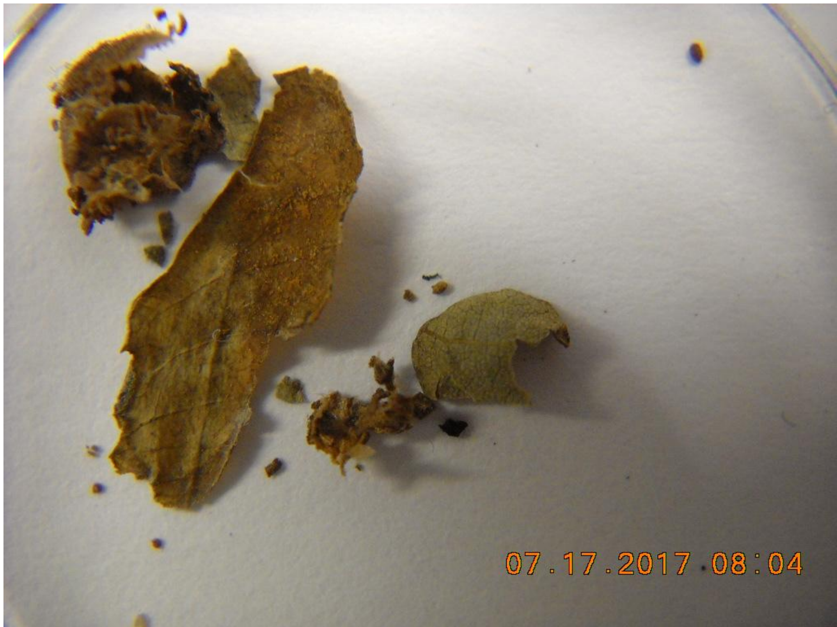
Photo 4 - FAA Digital Photograph. View of the organic material removed from Right Fuel Tank Strainer
