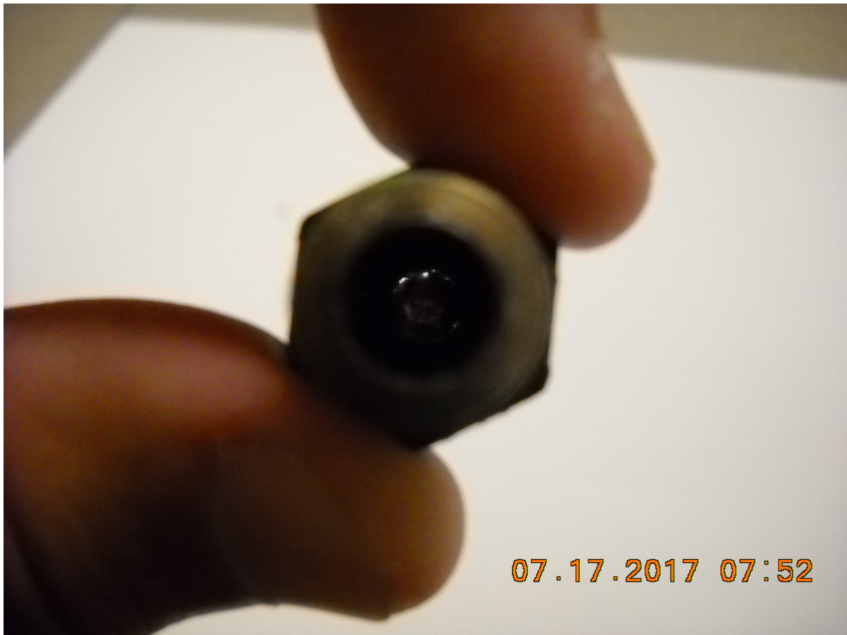
Photo 3 - FAA Digital Photograph. View of the near complete blockage of the Right Fuel Tank Strainer
