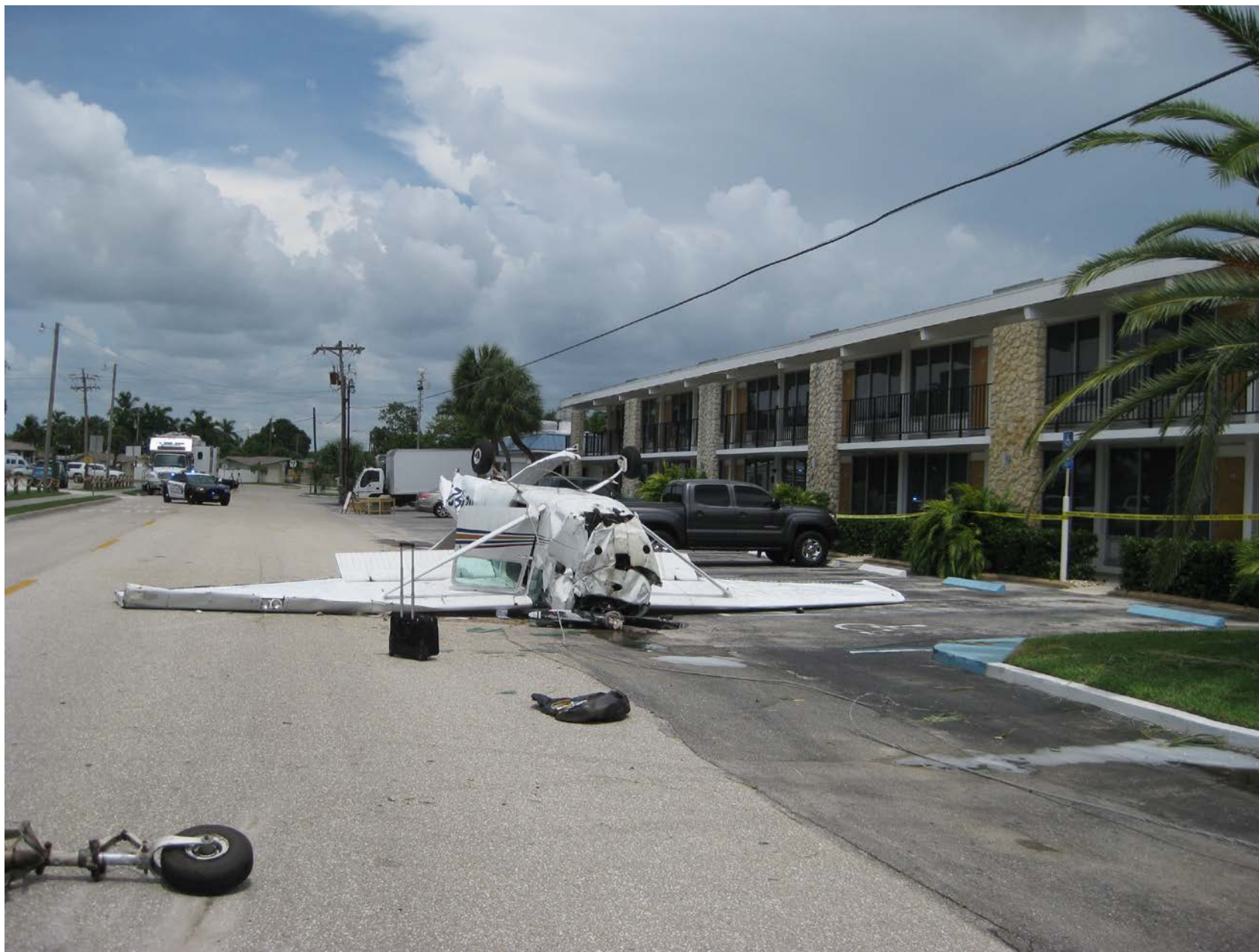
Photo 1 – View of main wreckage inverted in parking lot showing nose damage. (Courtesy of the FAA)
