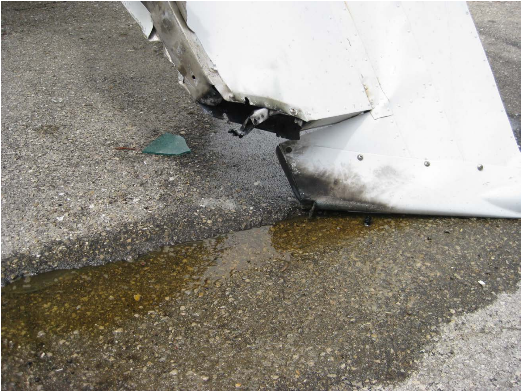
Photo 2 – View of fuel and water mixture that leaked from right wing.(Courtesy of the FAA)
