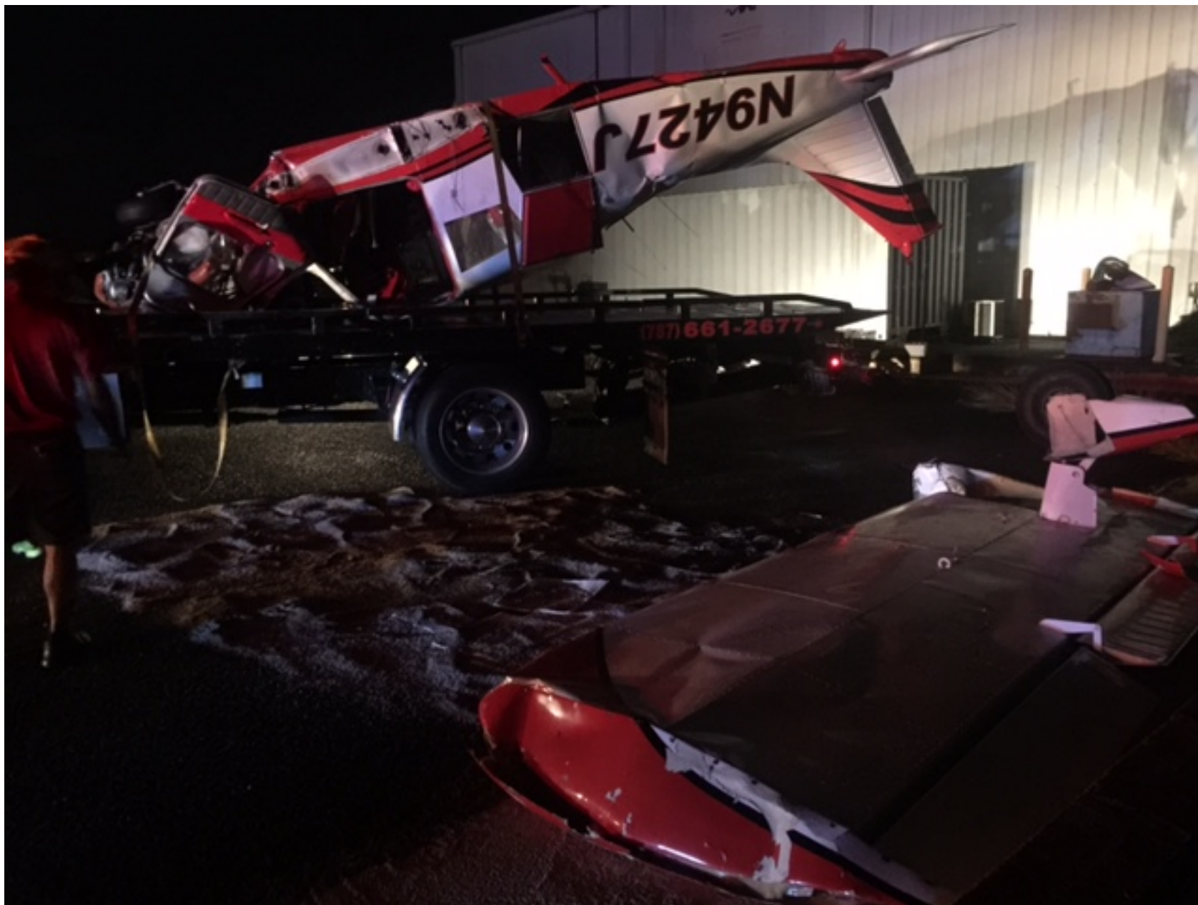
Photo 2 – Main Wreckage Recovered (Photo Courtesy of FAA)
