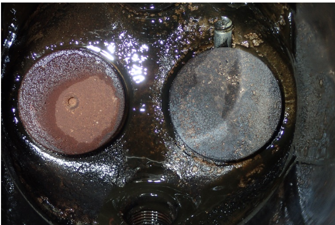
#2 Intake and Exhaust Valves with Debris
