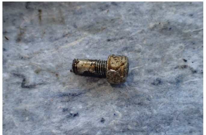
Bolt and nut found between the #2 intake valve head and seat
