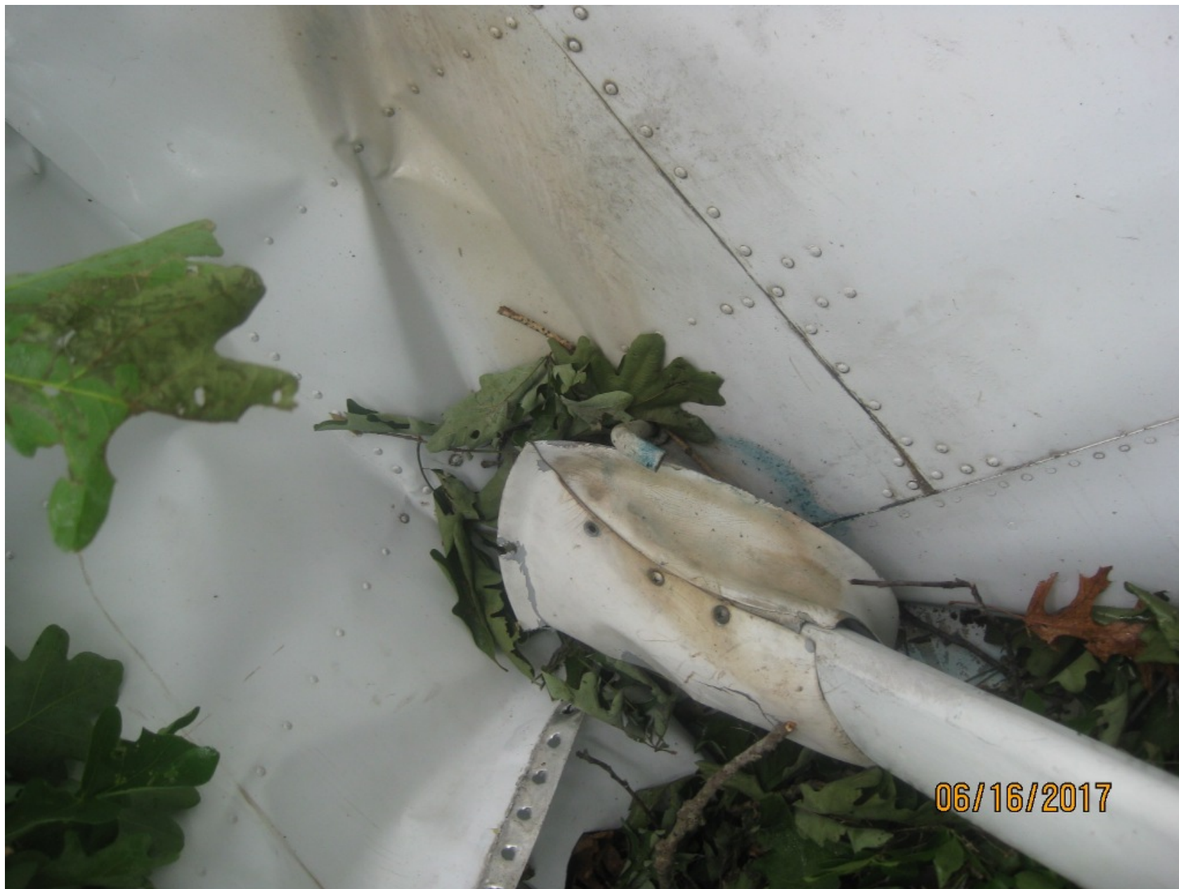
Photo 3 - FAA Digital Photograph. View of Portion of the Lower Surface of the Left Wing. Note the blue Stain at the Fuel Vent Line and on Lower Wing Skin near Fuel Vent Line.
