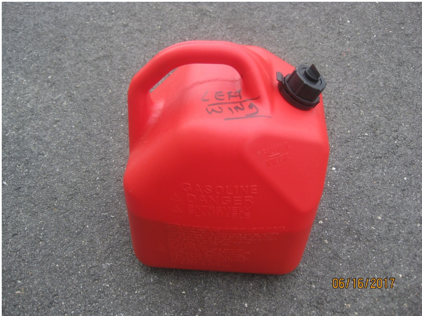
Photo 8 - FAA Digital Photograph. View Depicting the Approximately 2.5 gallons of Fuel Drained from the breached Left Fuel Tank
