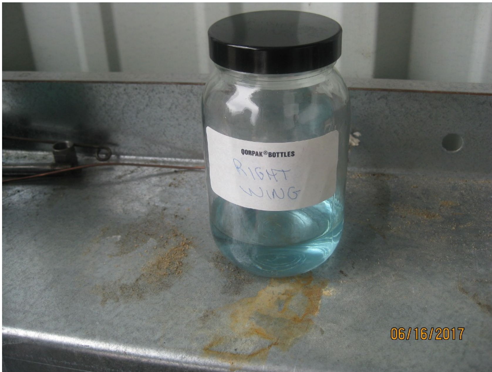
Photo 7 - FAA Digital Photograph. View Depicting the Approximately 6 ounces of Fuel Drained from the Un-breached Right Fuel Tank.
