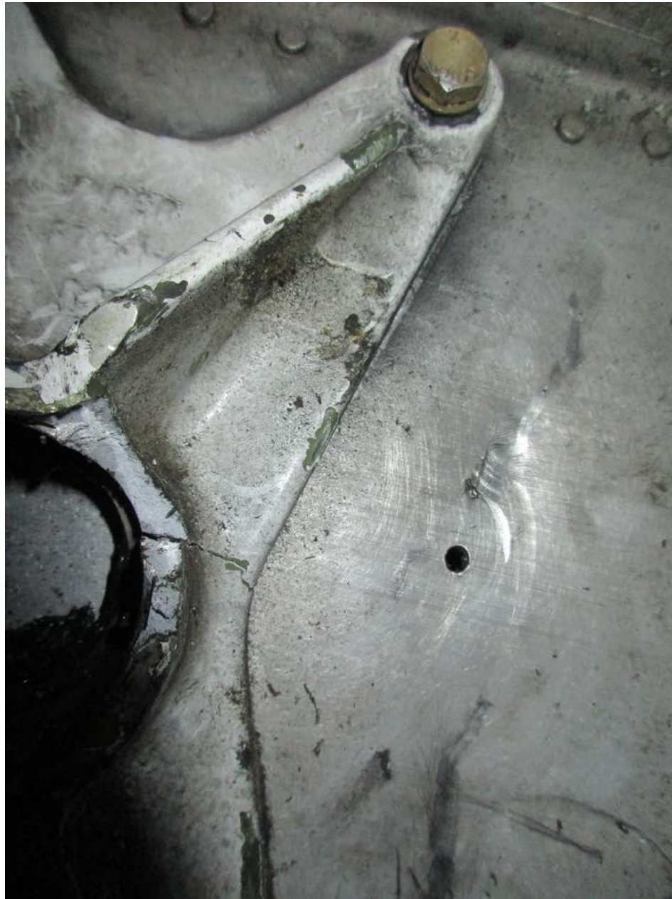
Photo 3 – Close up of fracture surface of trunnion
