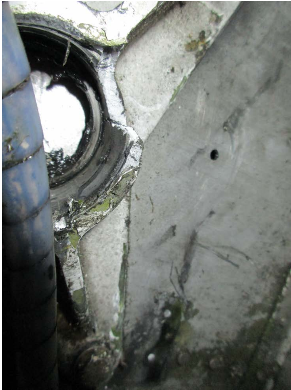
Photo 2 – View of top of the fracture surface of the trunnion
