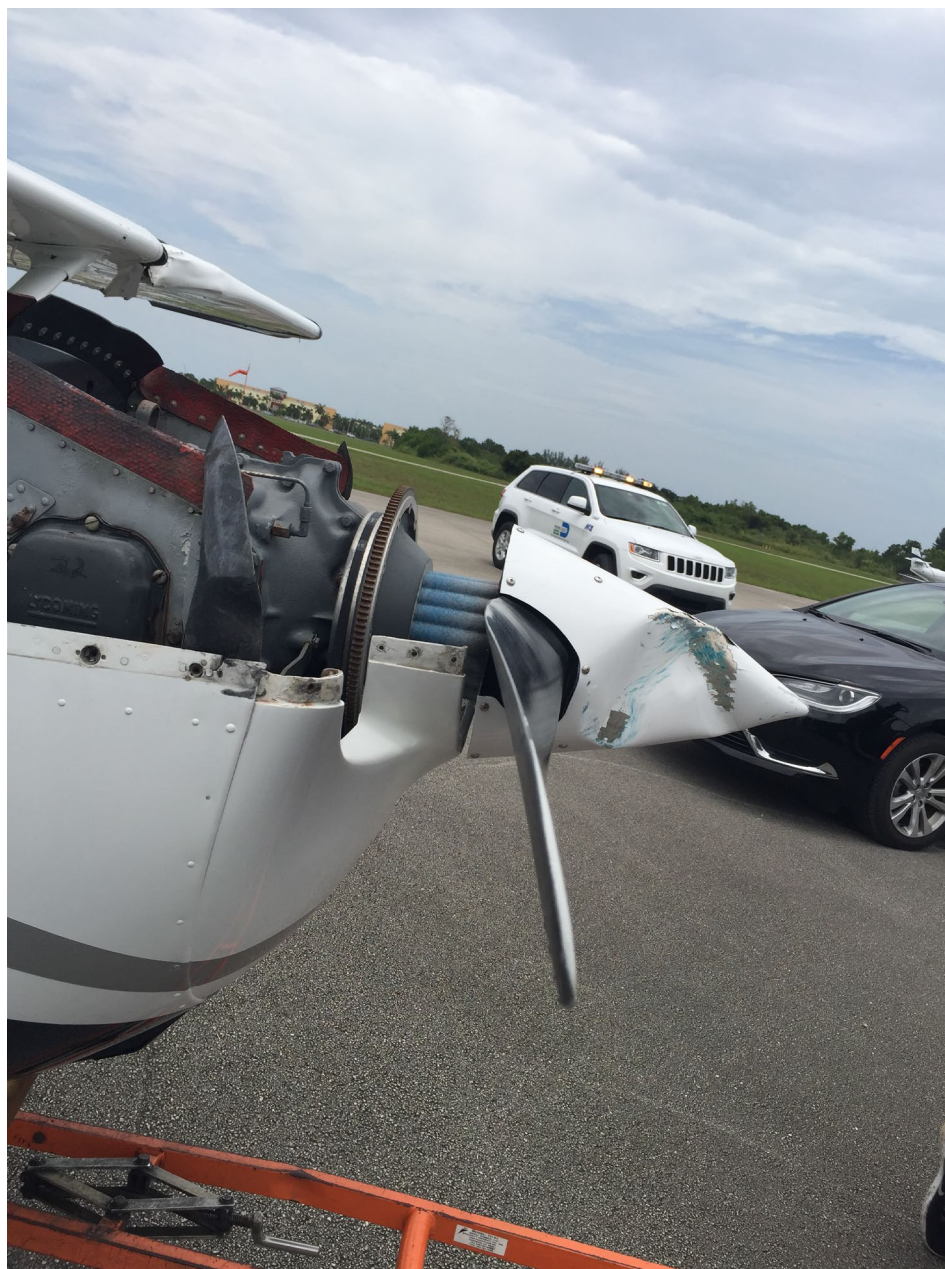
Photo 9 – Side View of Propeller Blade – Courtesy of FAA
