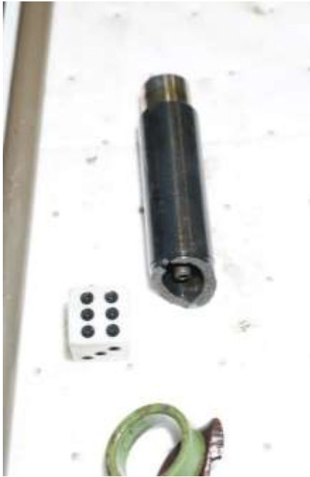
Picture 7. Fractured Exhaust Valve Lifter
