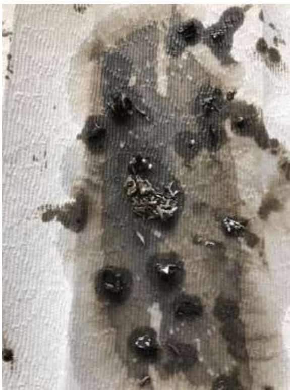
Figure 1 Metal remnants found in oil suction screen
