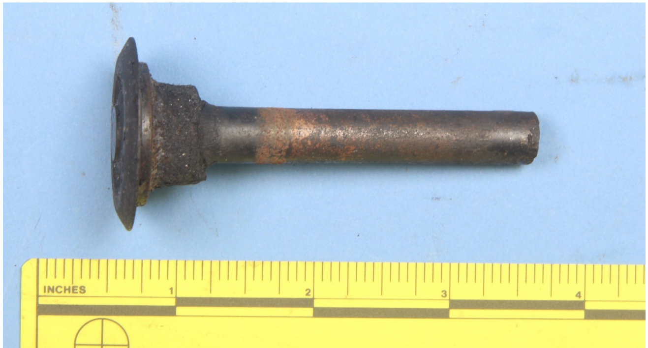
Figure 1 – The remnant of the exhaust valve, still affixed to the retainer, as received.
