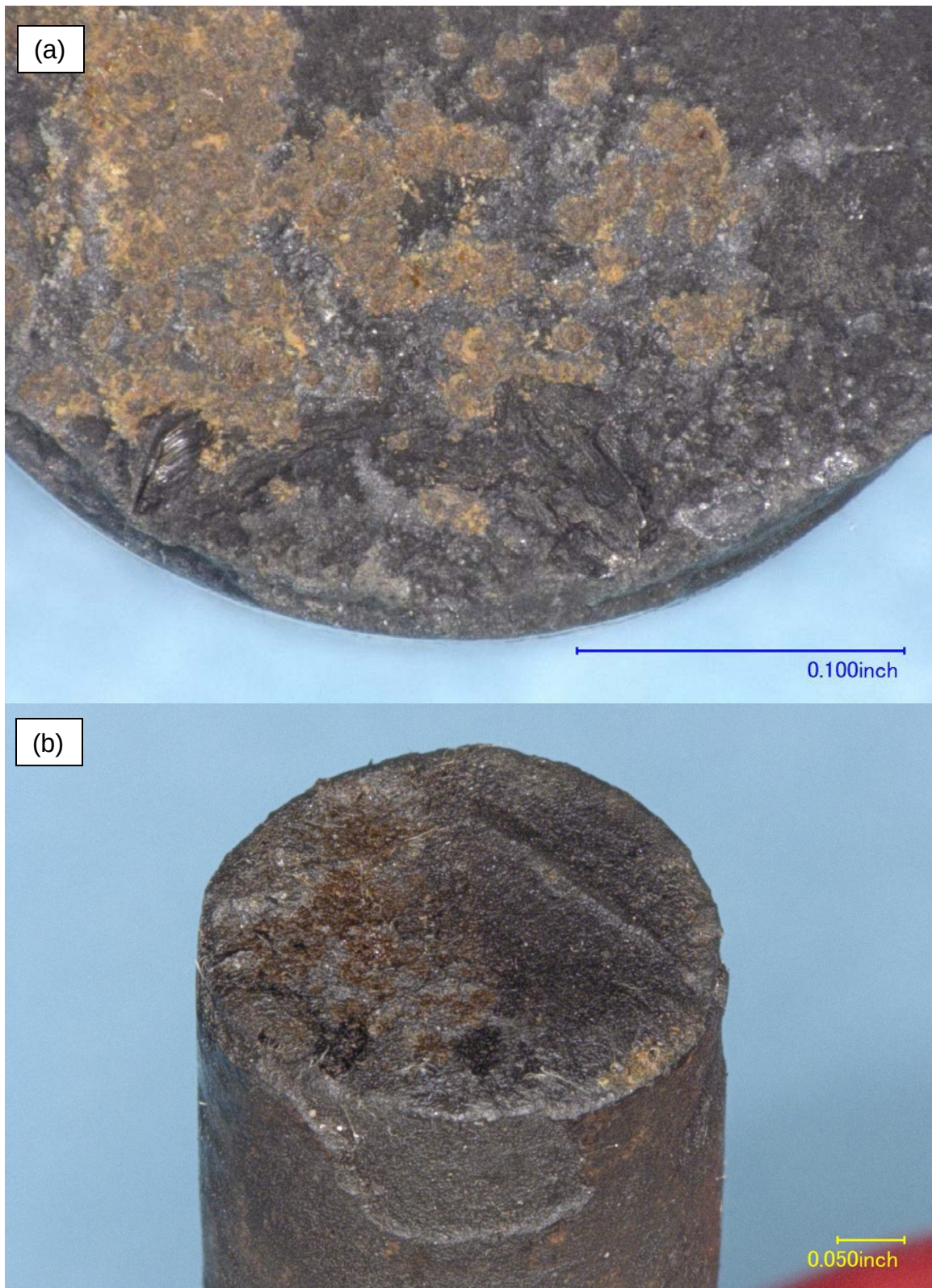
Figure 8 – The area consistent with the fatigue crack initiation site(s) viewed from (a) the fracture surface and (b) the side, showing outer material loss.
