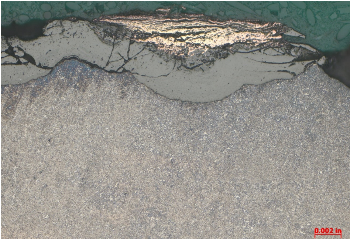
Figure 12 – BF micrograph of a transverse cross section of the valve stem near the fracture surface, showing surface oxidation (~200X, 2% Nital).
