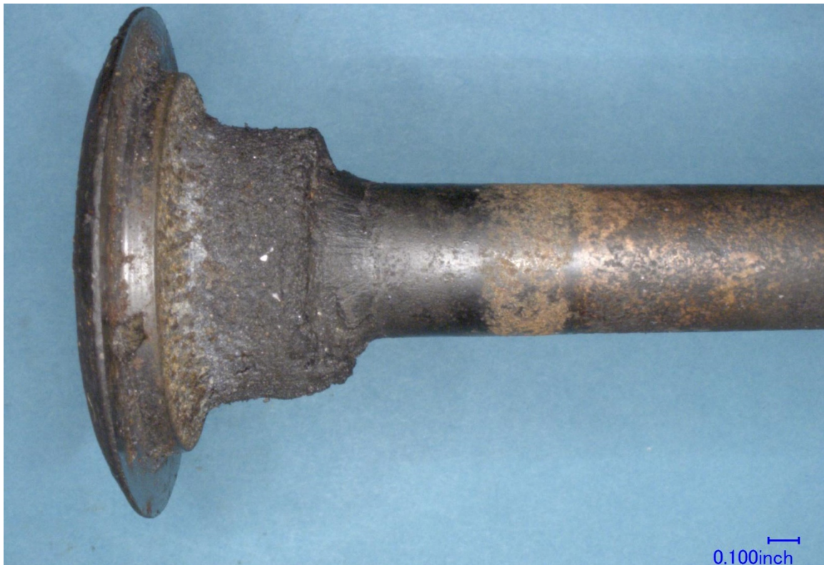
Figure 3 – The underside of the retainer on the exhaust valve, showing contamination buildup.
