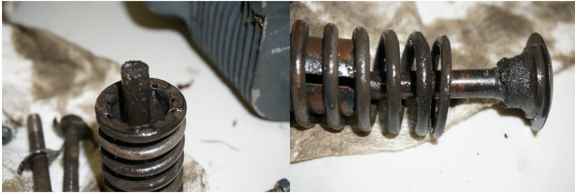
Picture 6. No. 4 Exhaust valve fractured stem and tip end
