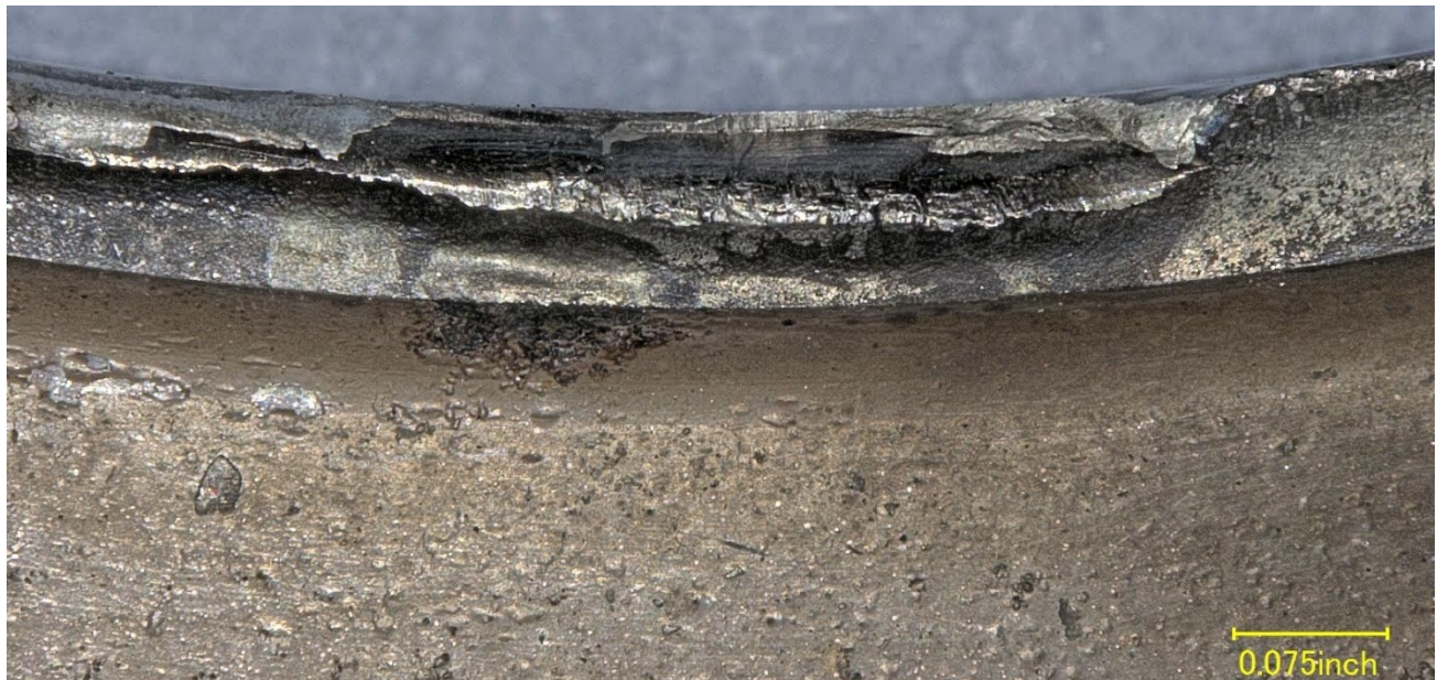
Figure 11 – Closer view of the initiation region from Figure 10.
