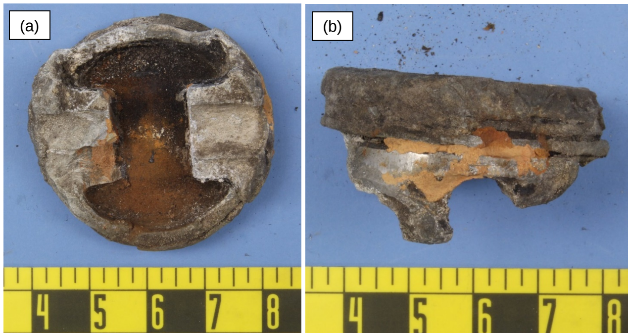
Figure 5 – The piston, as received, from (a) the underside and (b) the pin hole bore side.
