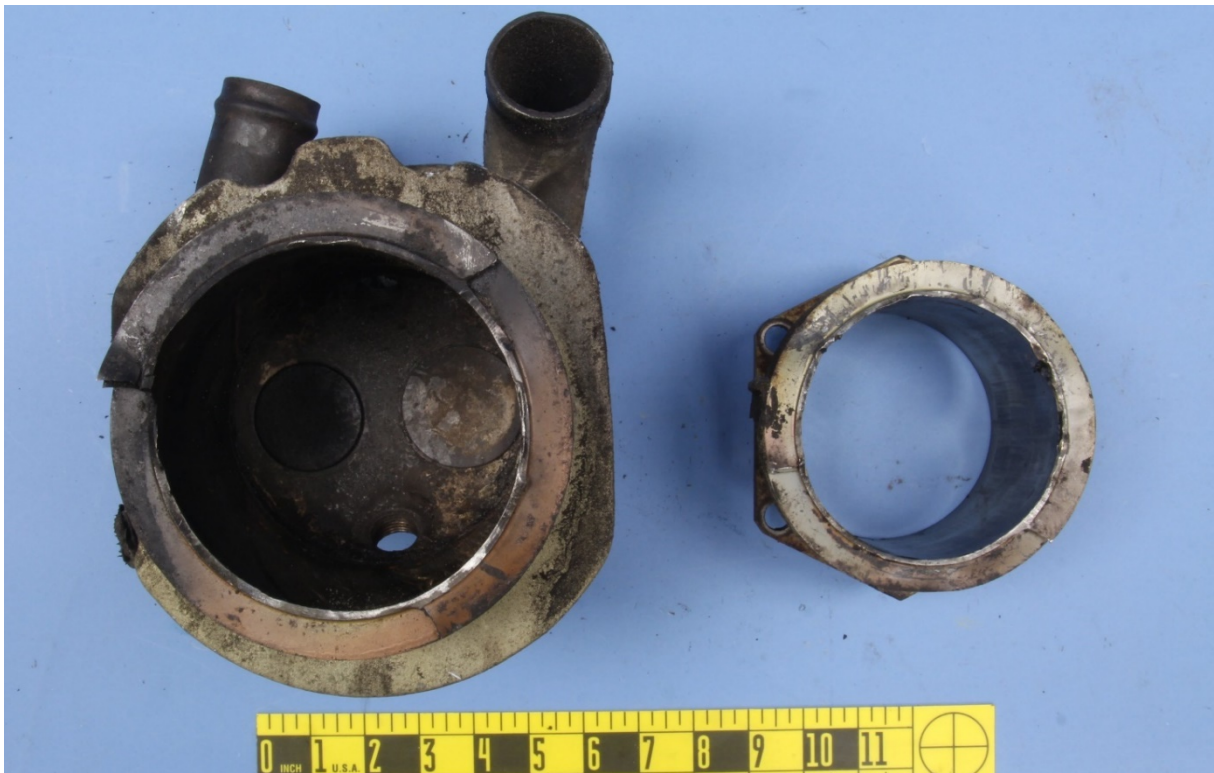
Figure 7 – The cylinder, as received, showing the mating fracture surfaces.
