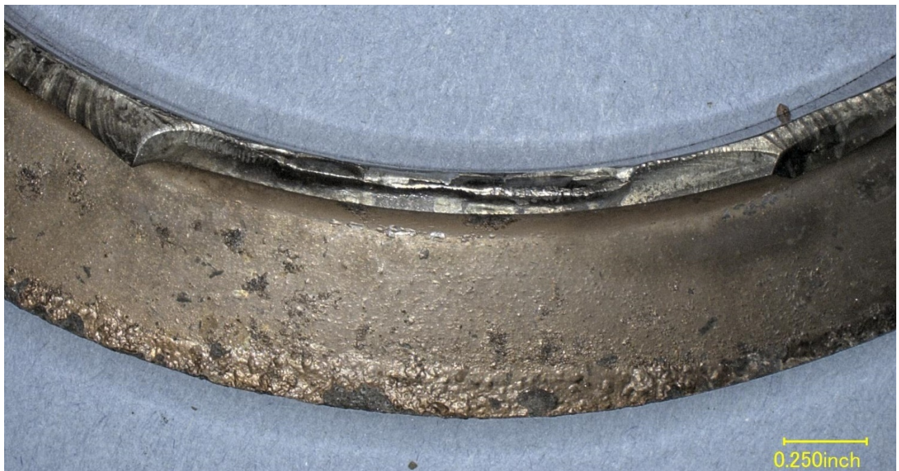
Figure 10 – Closer view of the initiation region of the cylinder fatigue crack, after sectioning and cleaning.
