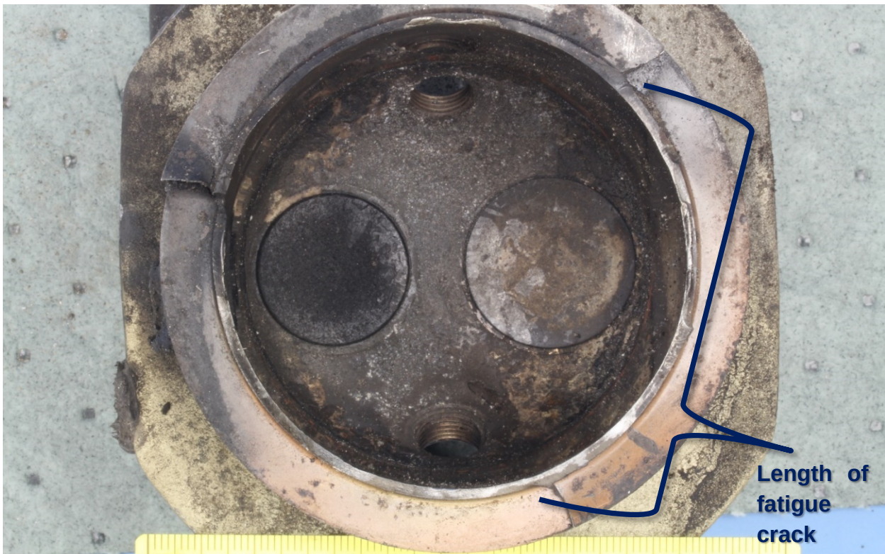
Figure 8 – The valve side of the cylinder, showing the fractured cylinder wall. The fatigue crack region is highlighted.
