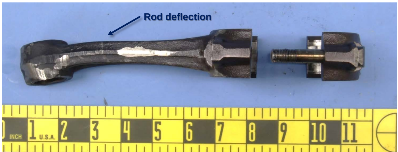
Figure 2 – The connecting rod pieces in Figure 1, shown from the side to demonstrate the deflection in the web.
