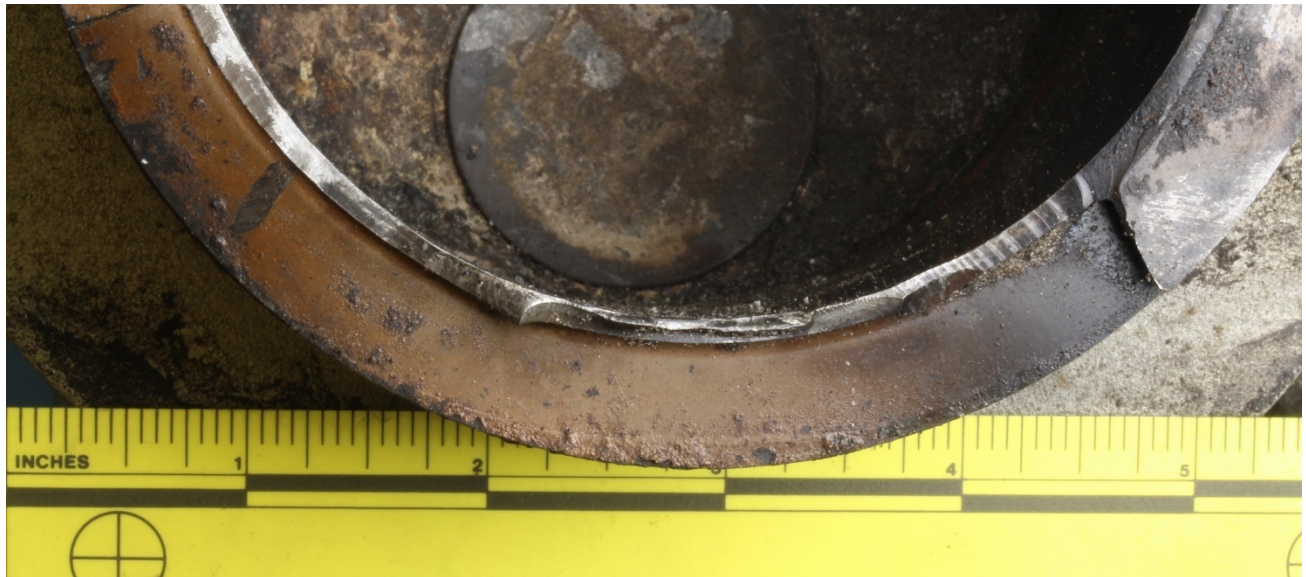
Figure 9 – Closer view of the fatigue crack wall of the cylinder from the on the valve-side half.
