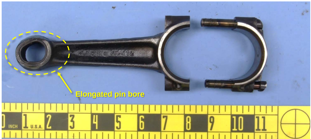
Figure 1 – The pieces of the connecting rod, as received. The elongated pin side is highlighted on the left.
