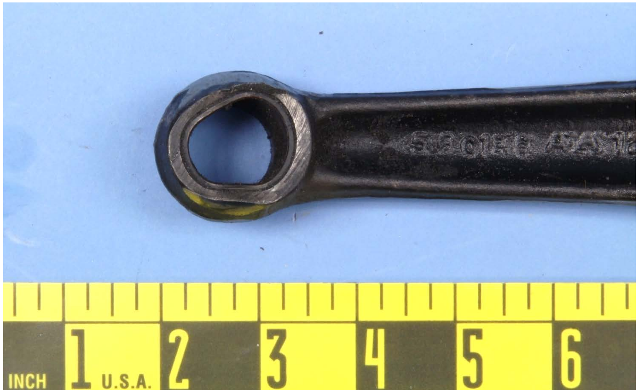
Figure 3 – A closer view of the elongated pin bore from Figure 1.
