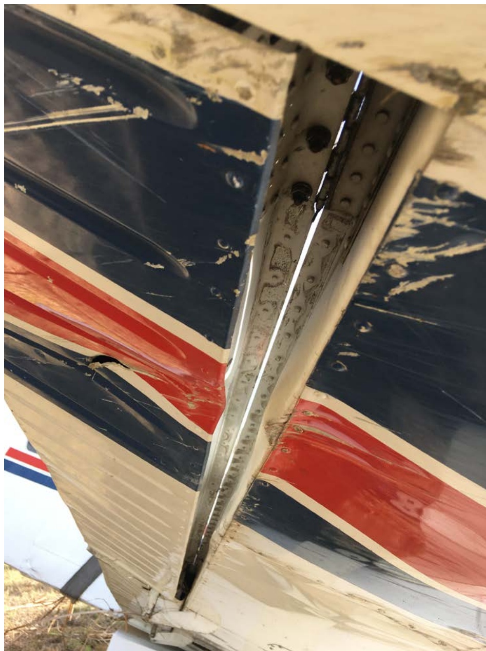
Photo 3 – View of damaged right aileron and wing spar
