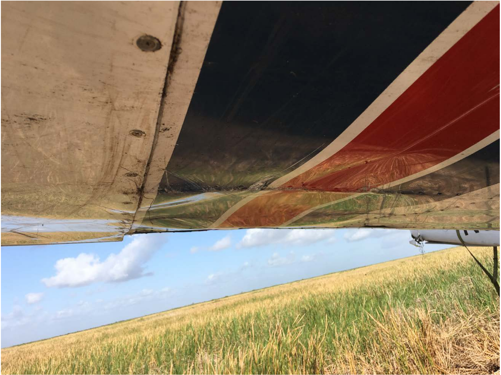
Photo 2 – View of damaged right wing spar
