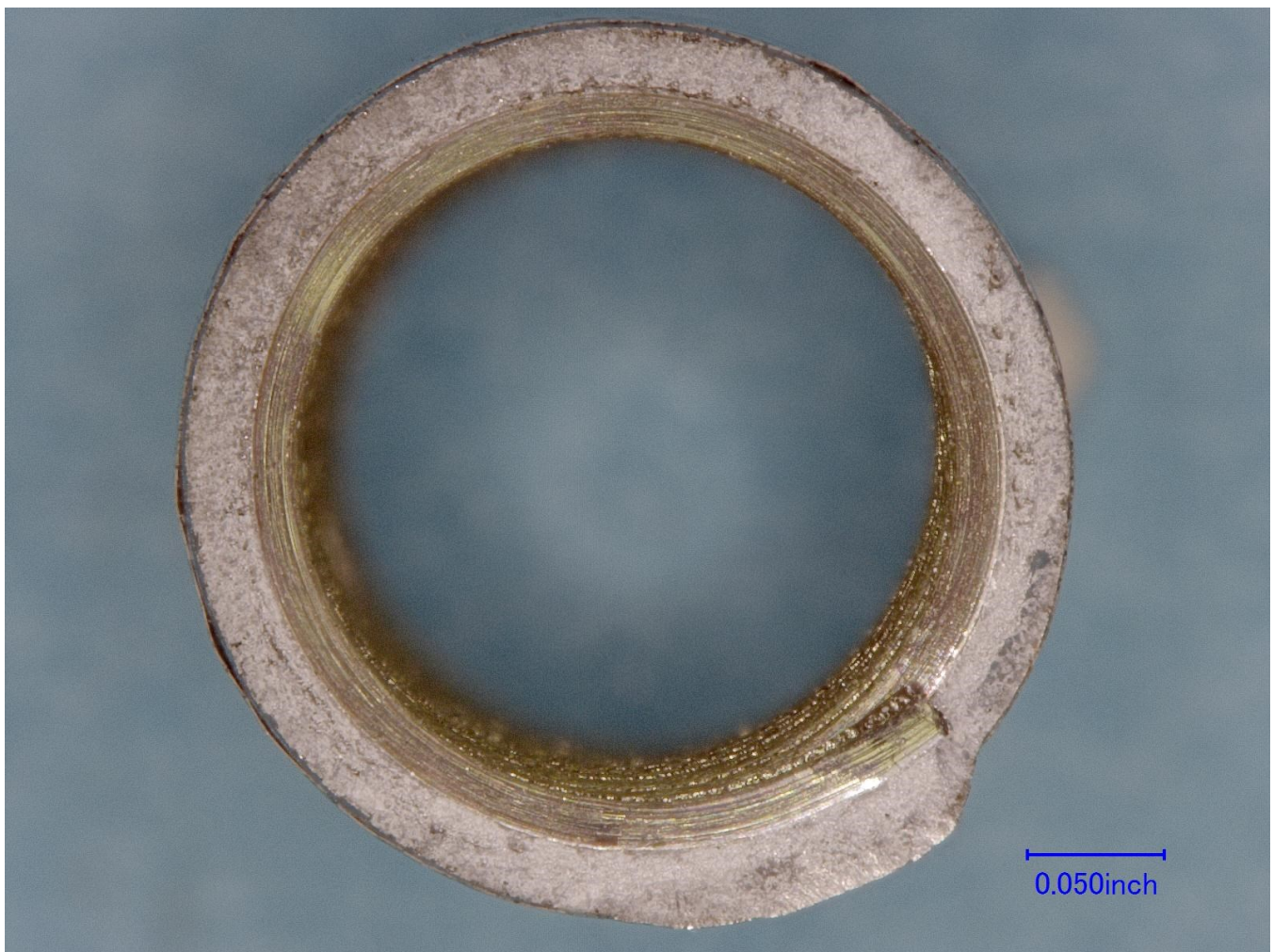
Figure 2 – The fracture surface from the shorter fragment of the broken tube.
