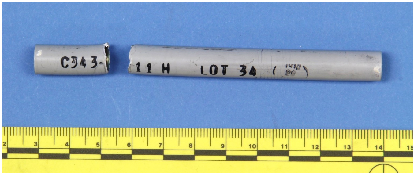
Figure 1 – The fractured anti-torque pedal control tube halves, as received.
