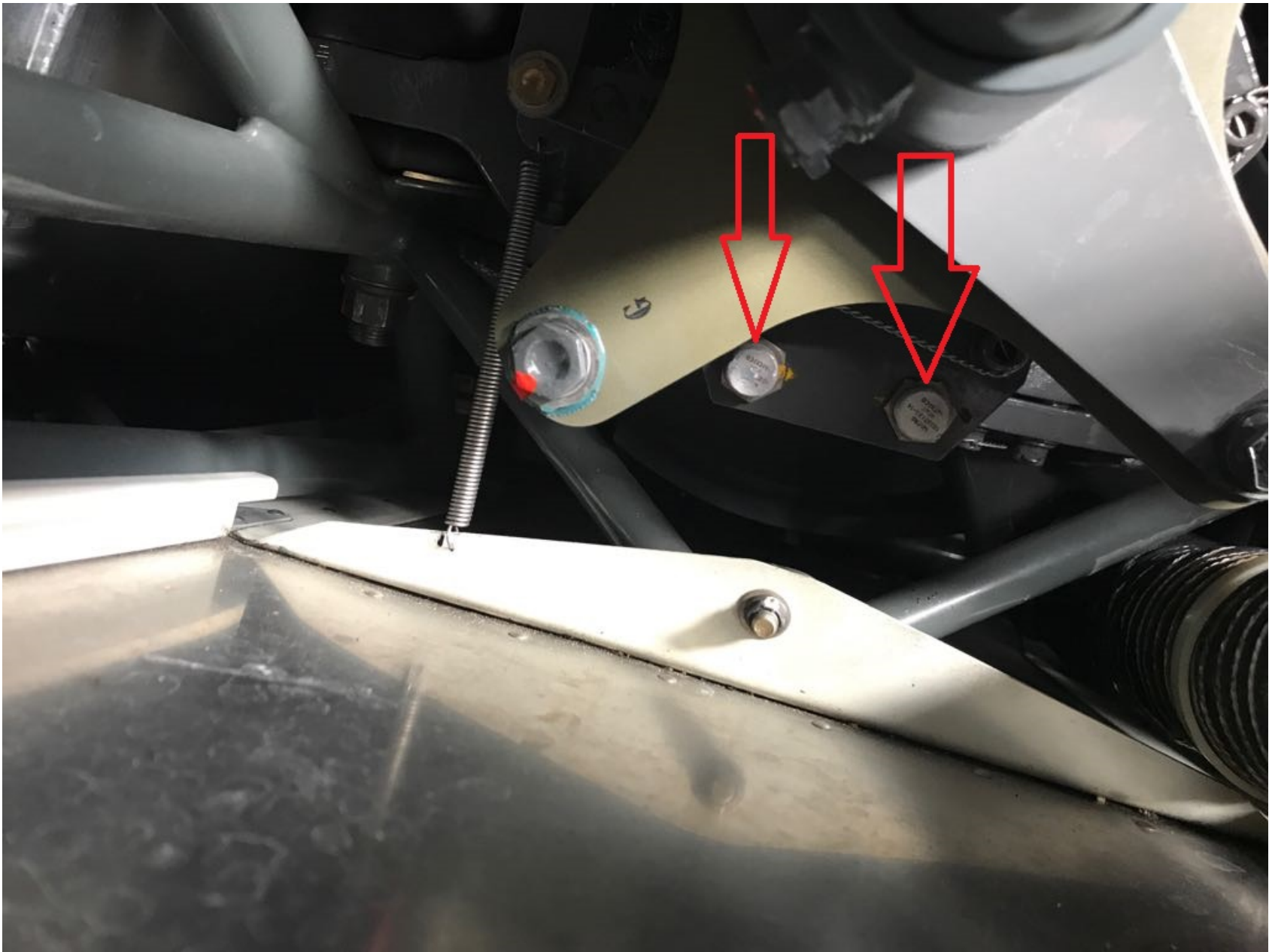
Photo 5 - Digital Photograph Provided by Operator. Red Arrows Points to Both Main Rotor RPM Sender Assemblies.
