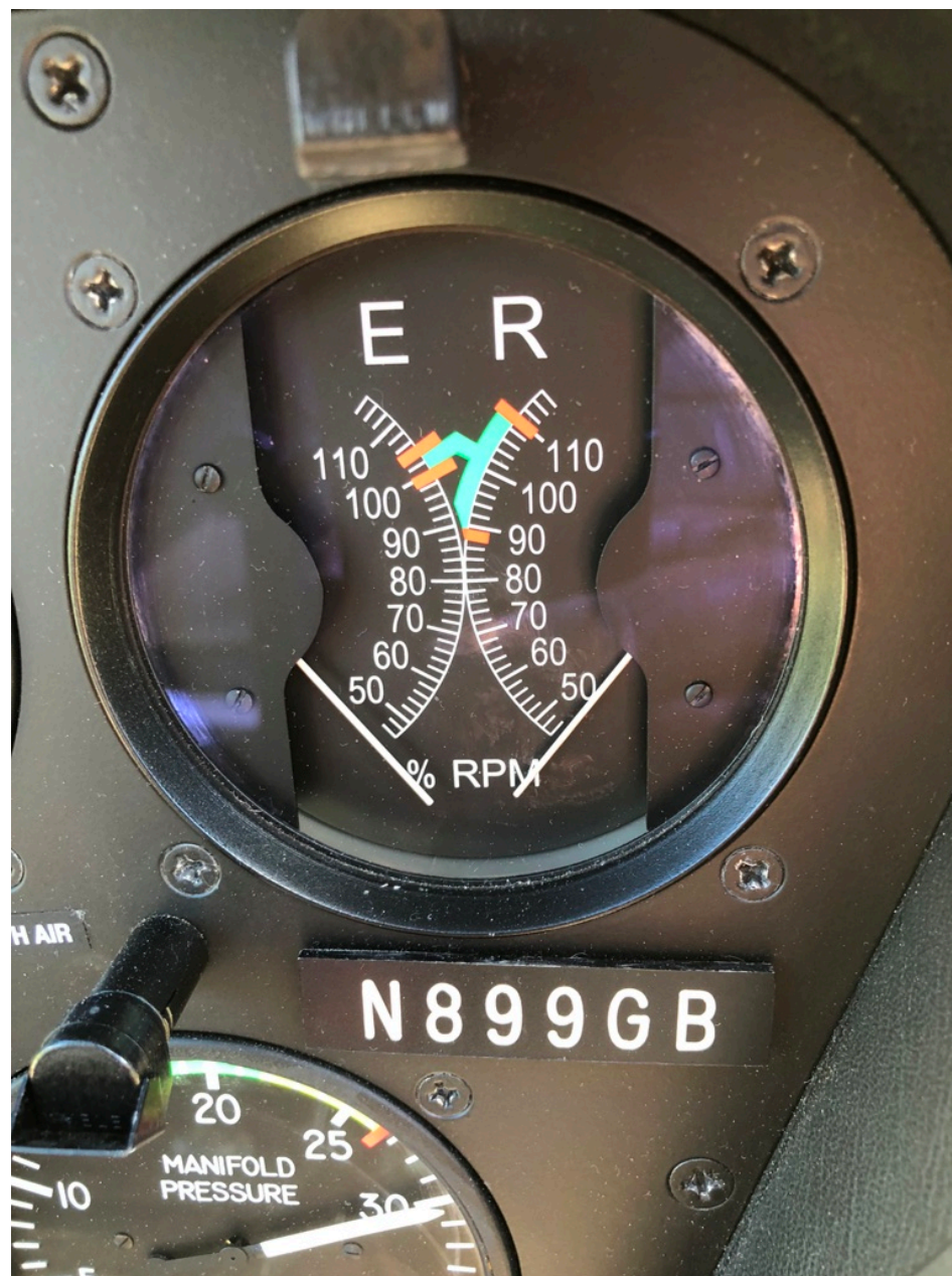
Photo 2 - Digital Photograph Provided by Operator. View of the Dual Tachometer. Note the Lowest Numeric Marking of 50 on the Main Rotor.
