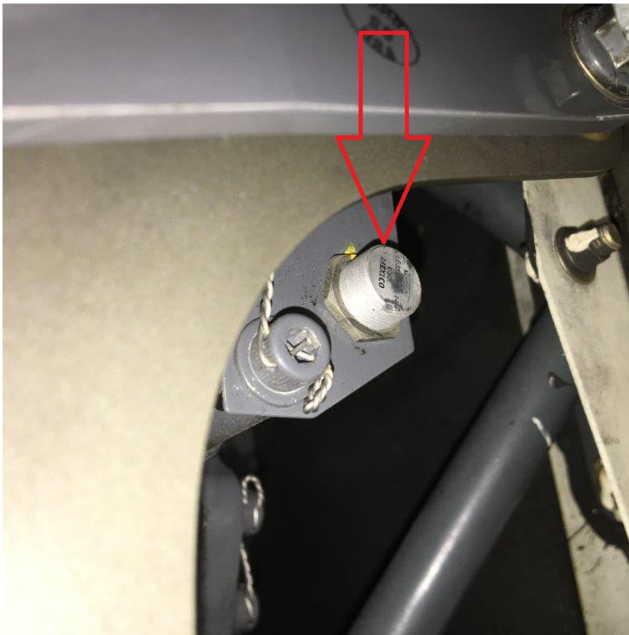
Photo 6 - Digital Photograph Provided by FAA. Close-Up View. Red Arrow Points to 1 damaged Main Rotor RPM Sender Assembly.
