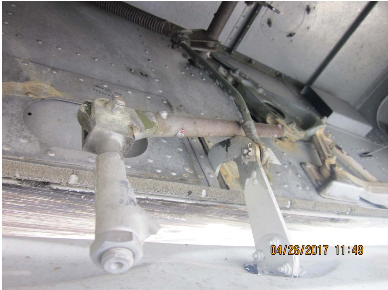
Photo 6 – Nose landing gear broken retract mechanism. (Courtesy of FAA)
