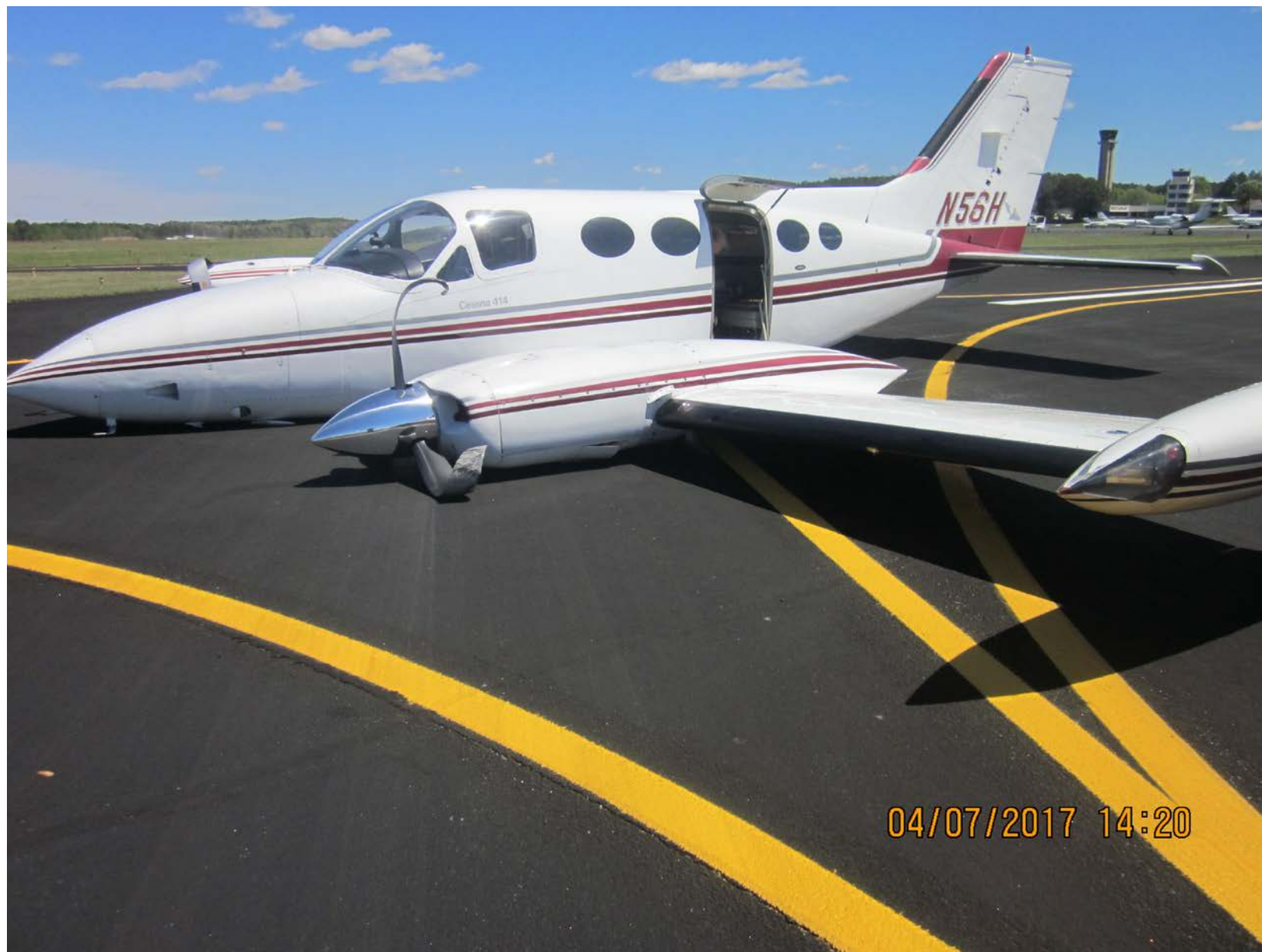
Photo 1 – Left front view of airplane showing propeller damage. (Courtesy of FAA)
