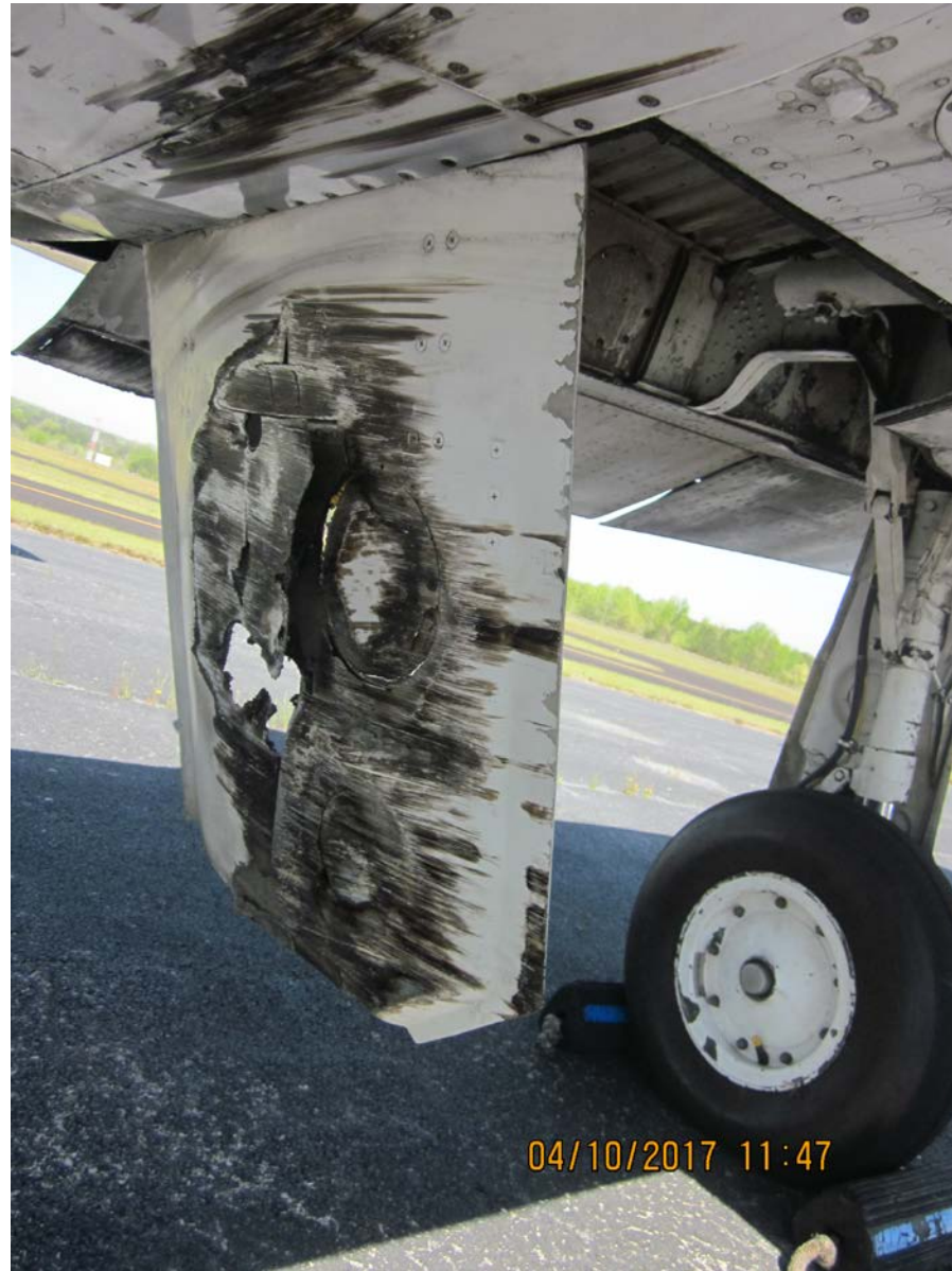
Photo 5 – Left main landing gear and door damage. (Courtesy of FAA)
