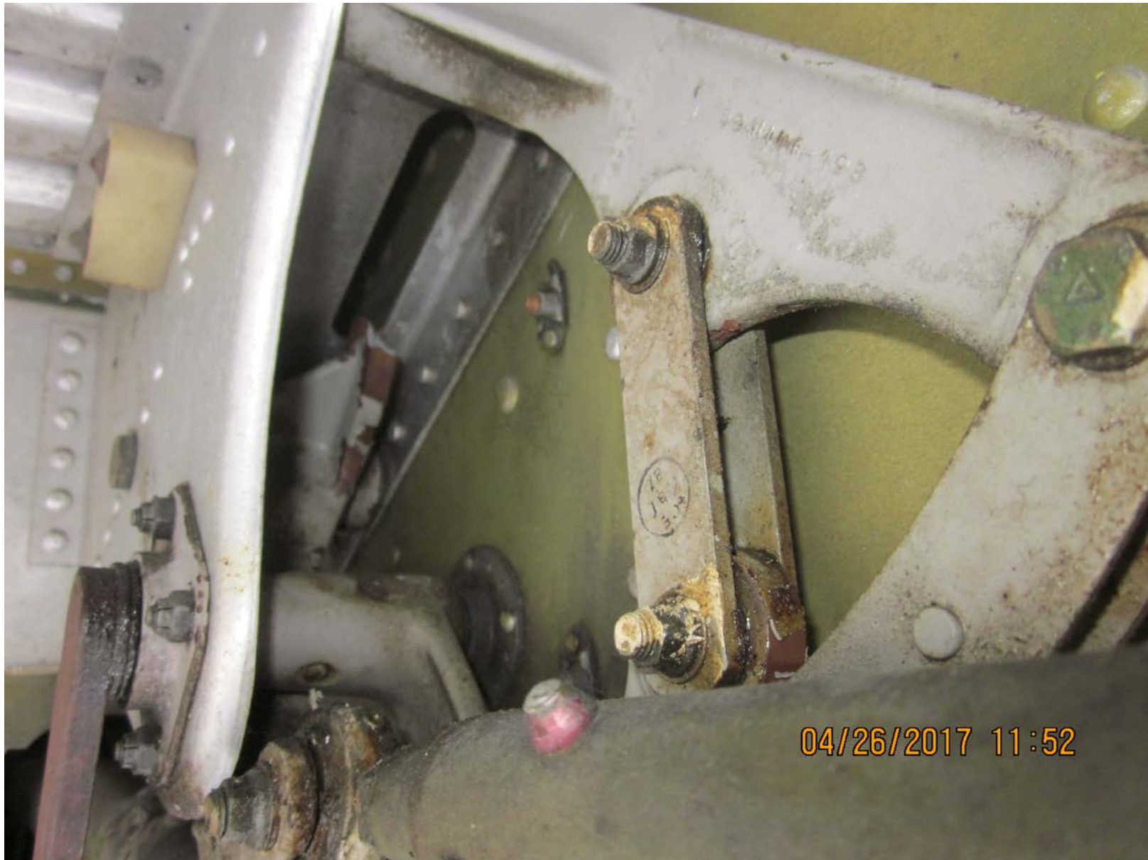
Photo 7 – Right main landing gear retract mechanism break. (Courtesy of FAA)
