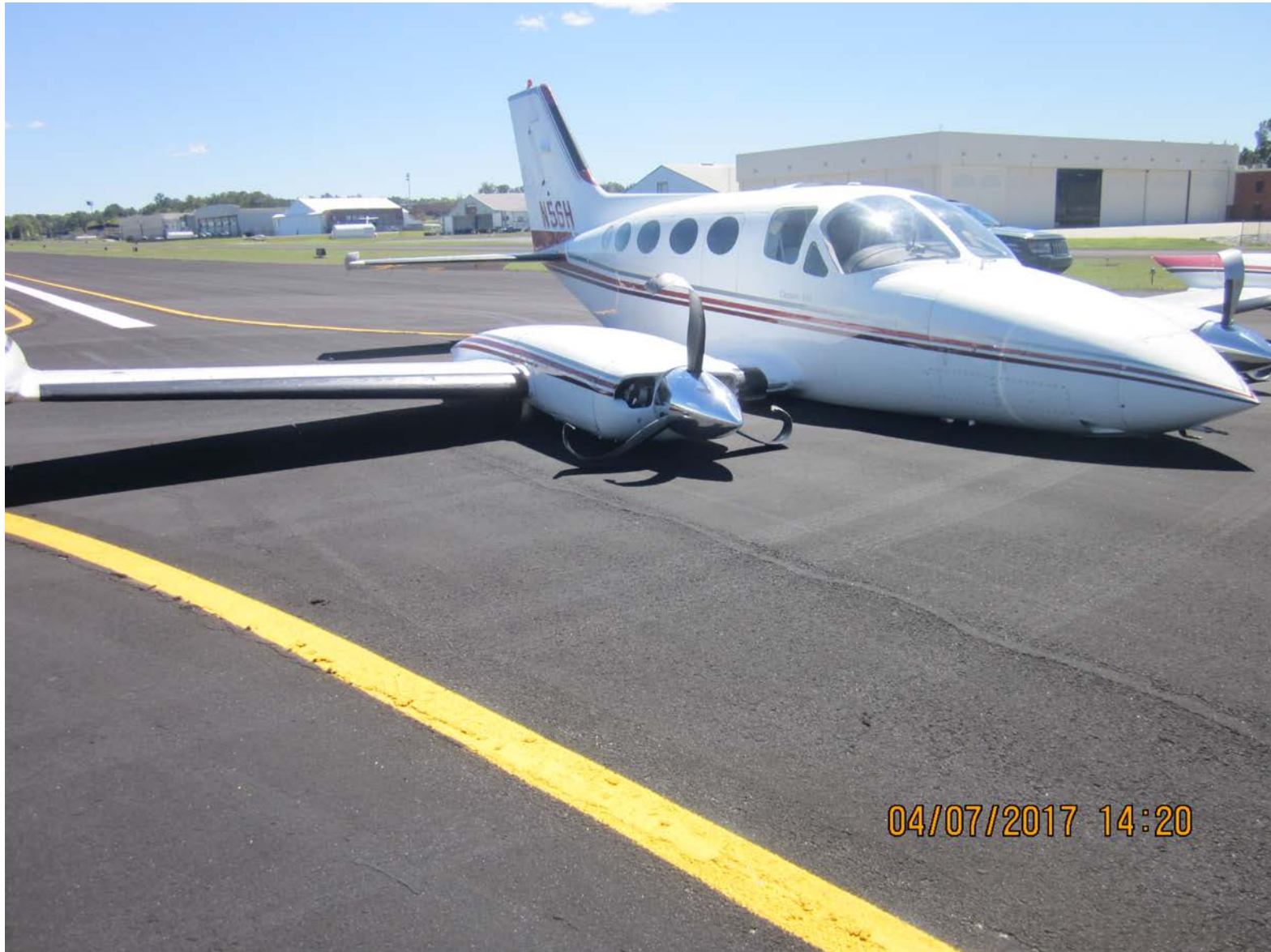
Photo 2 – Right front quarter view of airplane showing propeller damage. (Courtesy of FAA)
