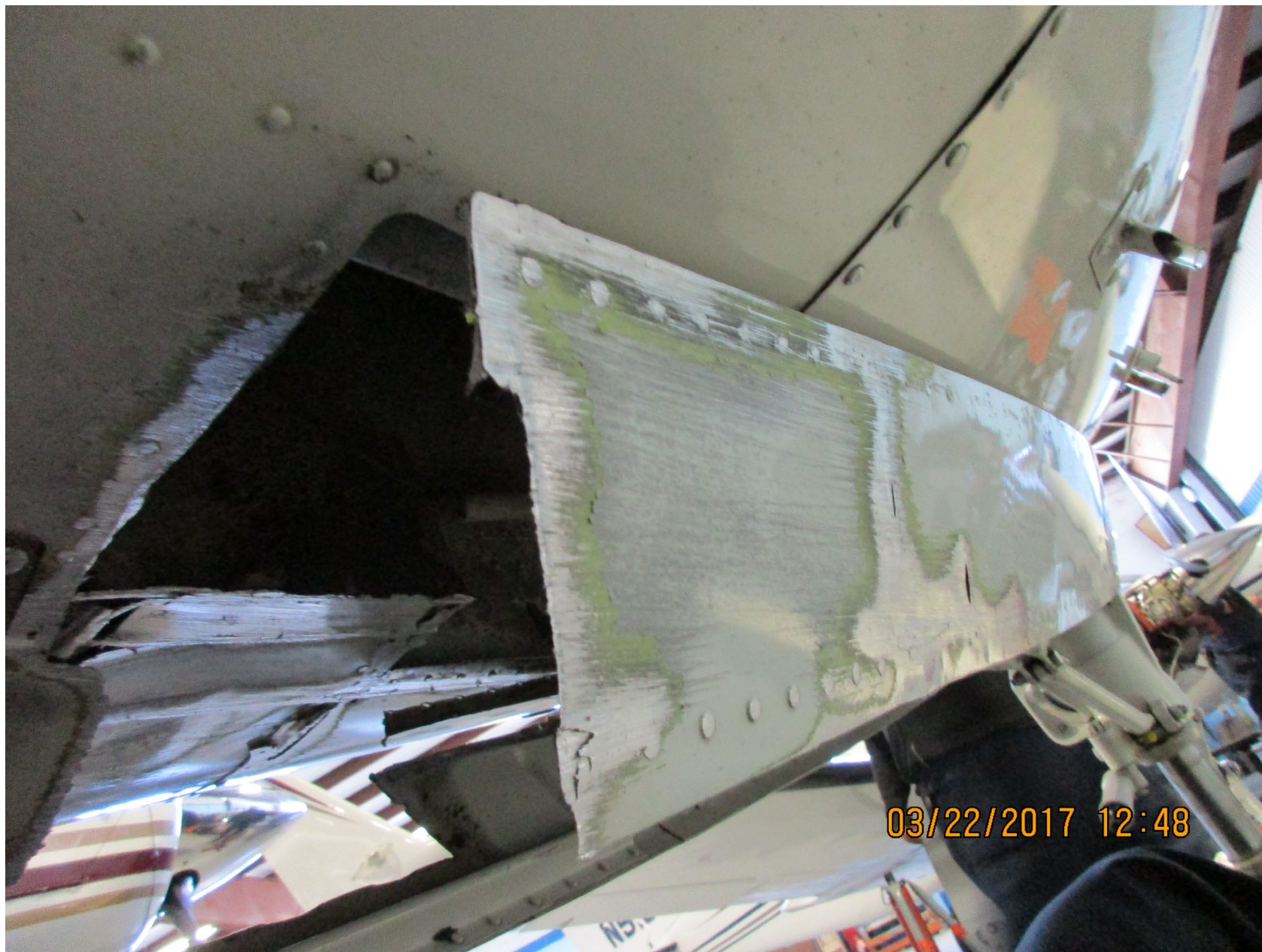
Photo 13 – Nose Landing Gear Door Right Side – Courtesy of FAA
