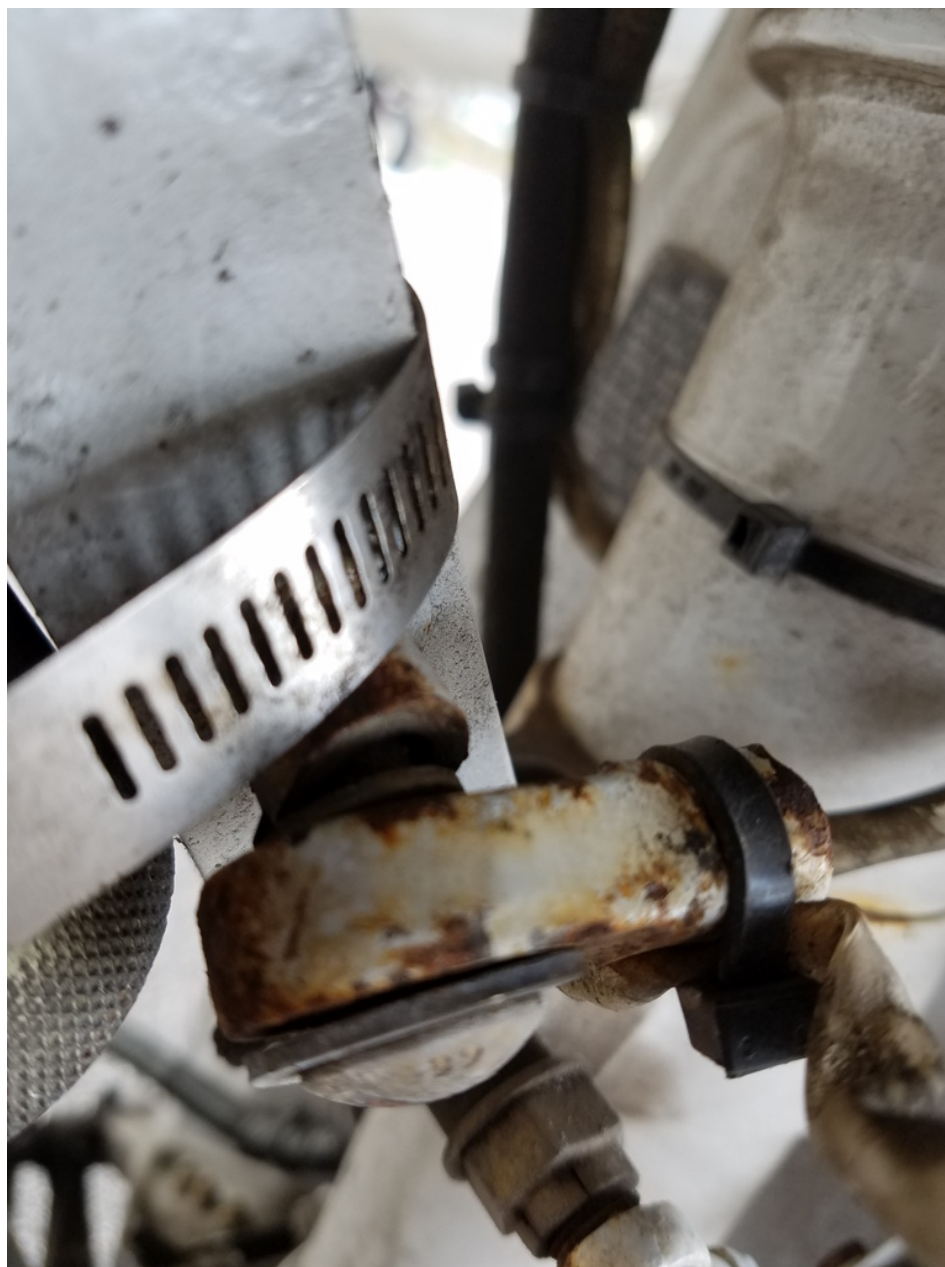
Photo 4 – Left Main Landing Gear Downlock Link (Photo Courtesy of FAA)
