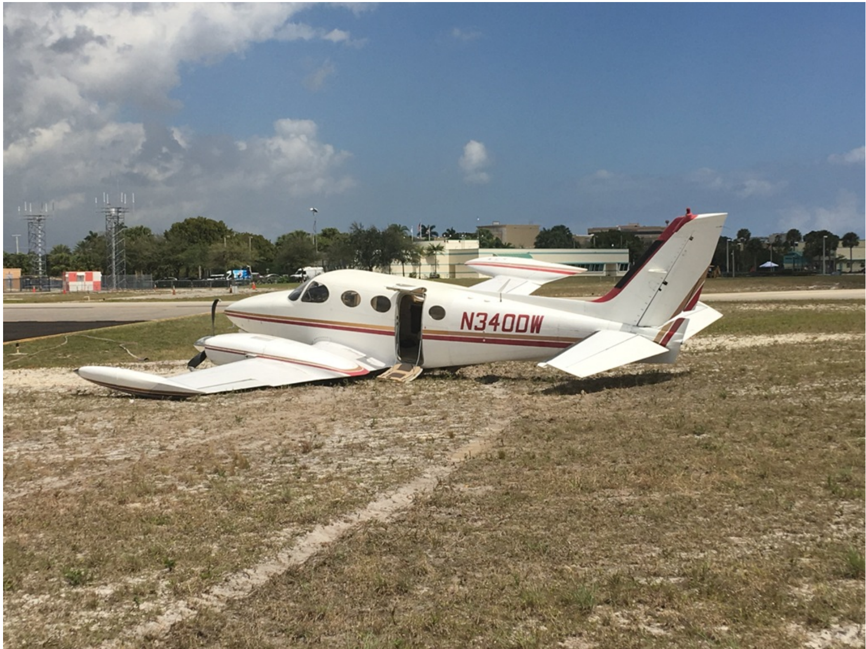
Photo 1 – Main Wreckage (Photo Courtesy of FAA)
