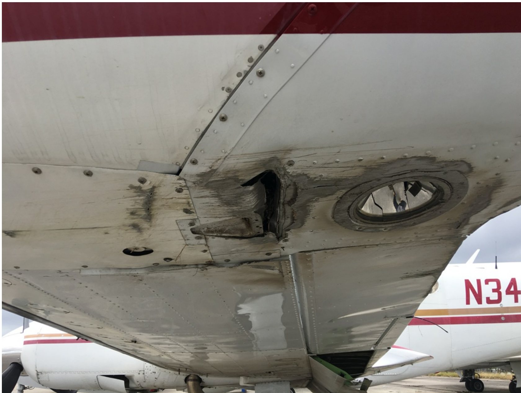
Photo 2 – Left Wing Damage (Photo Courtesy of FAA)
