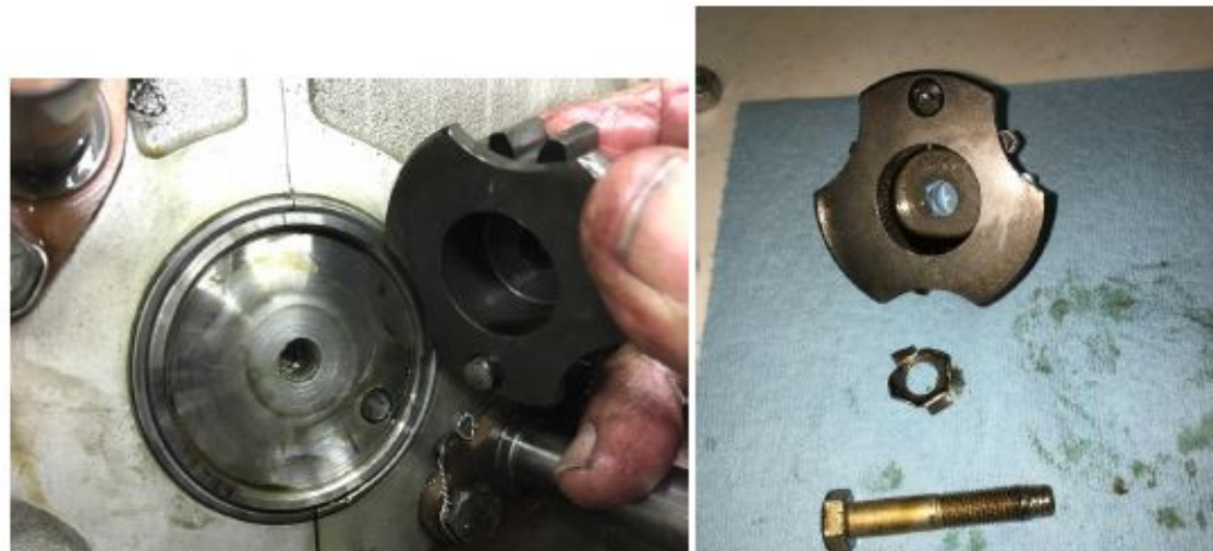
Photo 1 – Photograph of crankshaft gear bolt as found and post removal. Note damaged threads.
