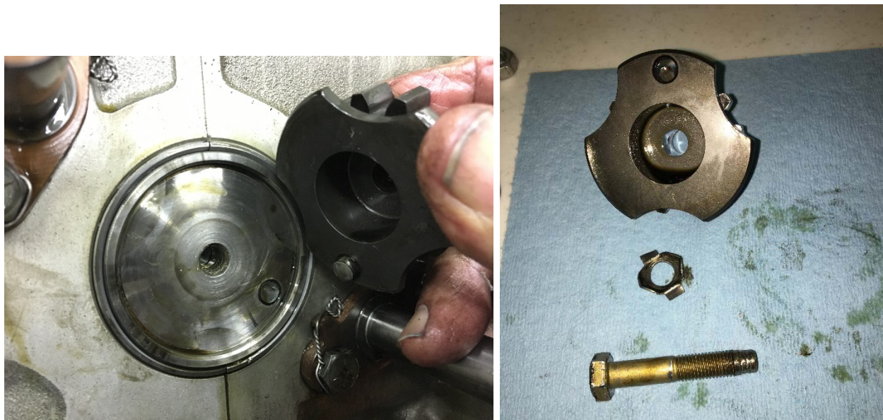
Picture 3. View of sheared pin and full crankshaft gear bolt.
