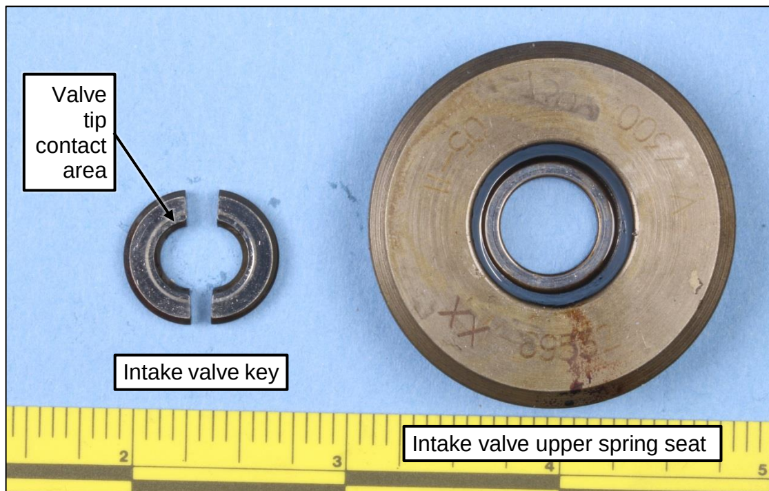
Figure 2. View of the outboard faces of the intake valve key and upper spring seat.
