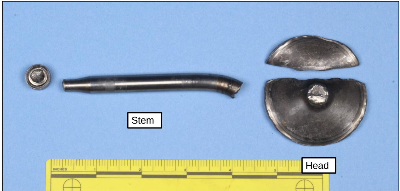
Figure 3. Overall view of the intake valve.
