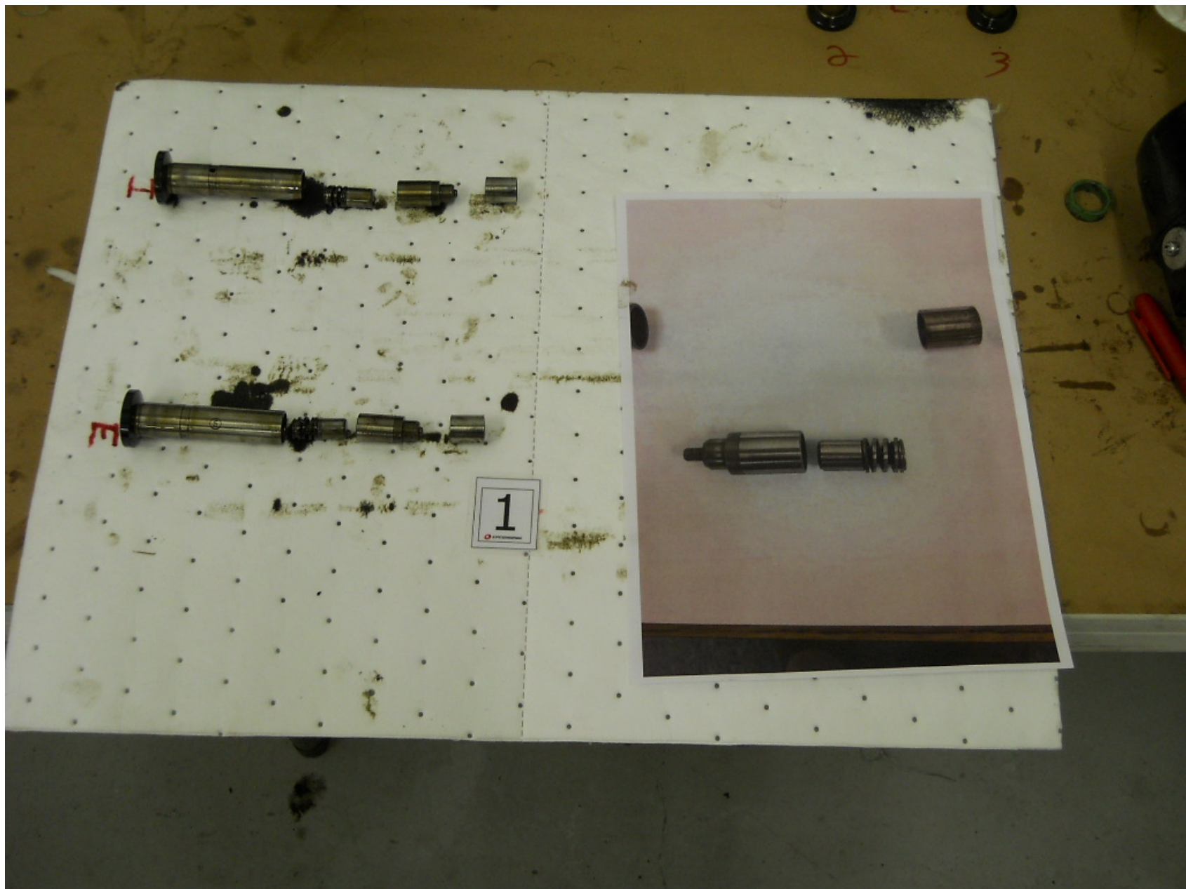
Photo 6 - #1 Cylinder Tappet Assembly (NTSB)
