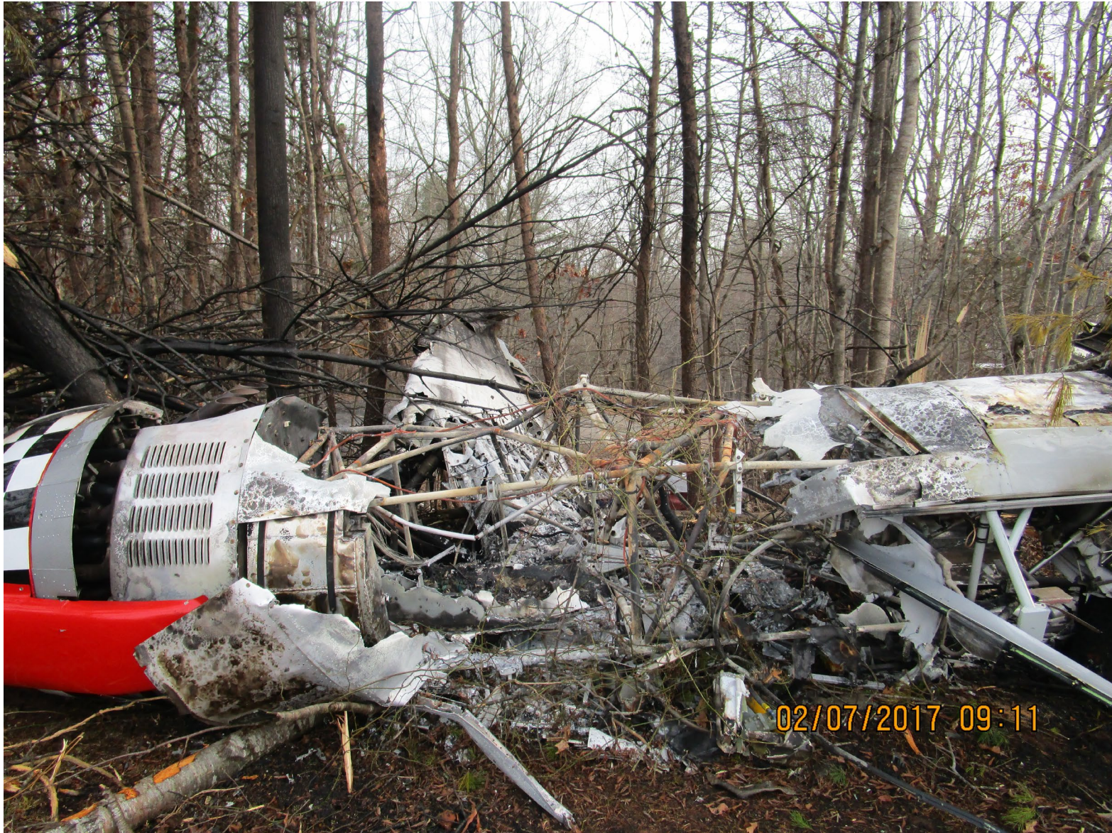
Photo 1 – View of overall wreckage of airplane showing impact and thermal damage. (Courtesy of FAA)
