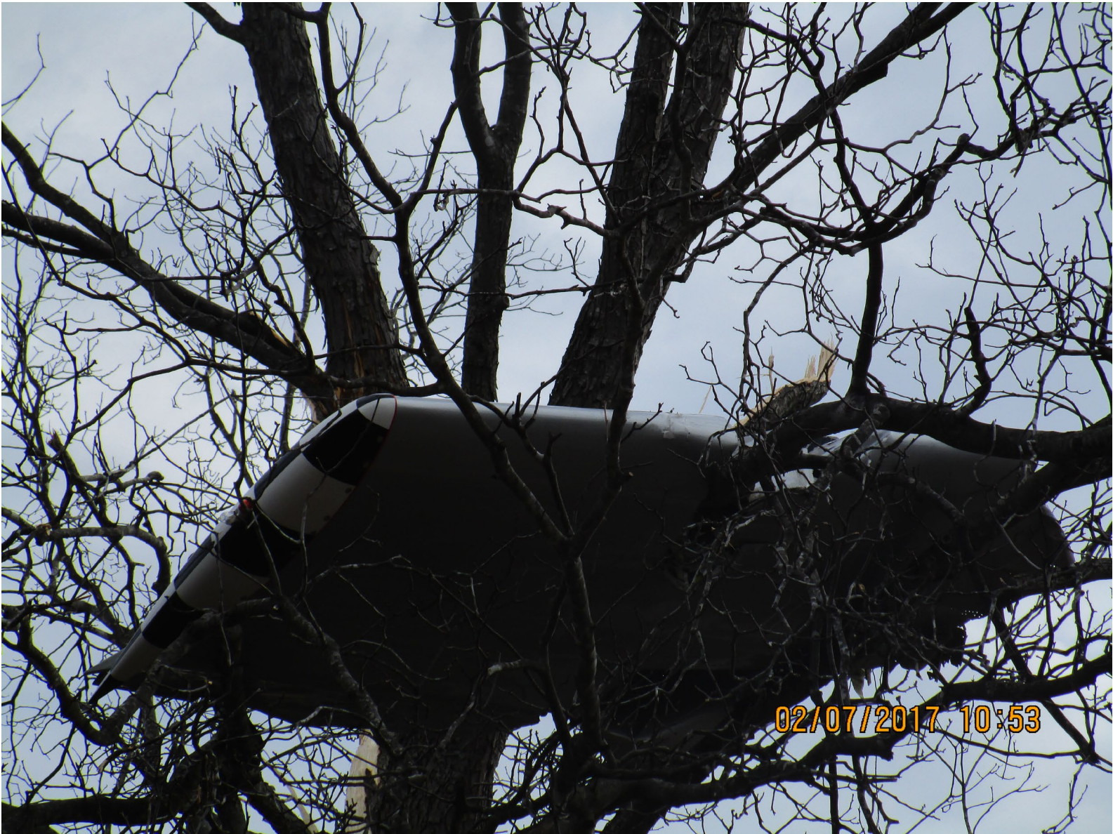
Photo 3 – View of separated wing located up in the trees. (Courtesy of FAA)
