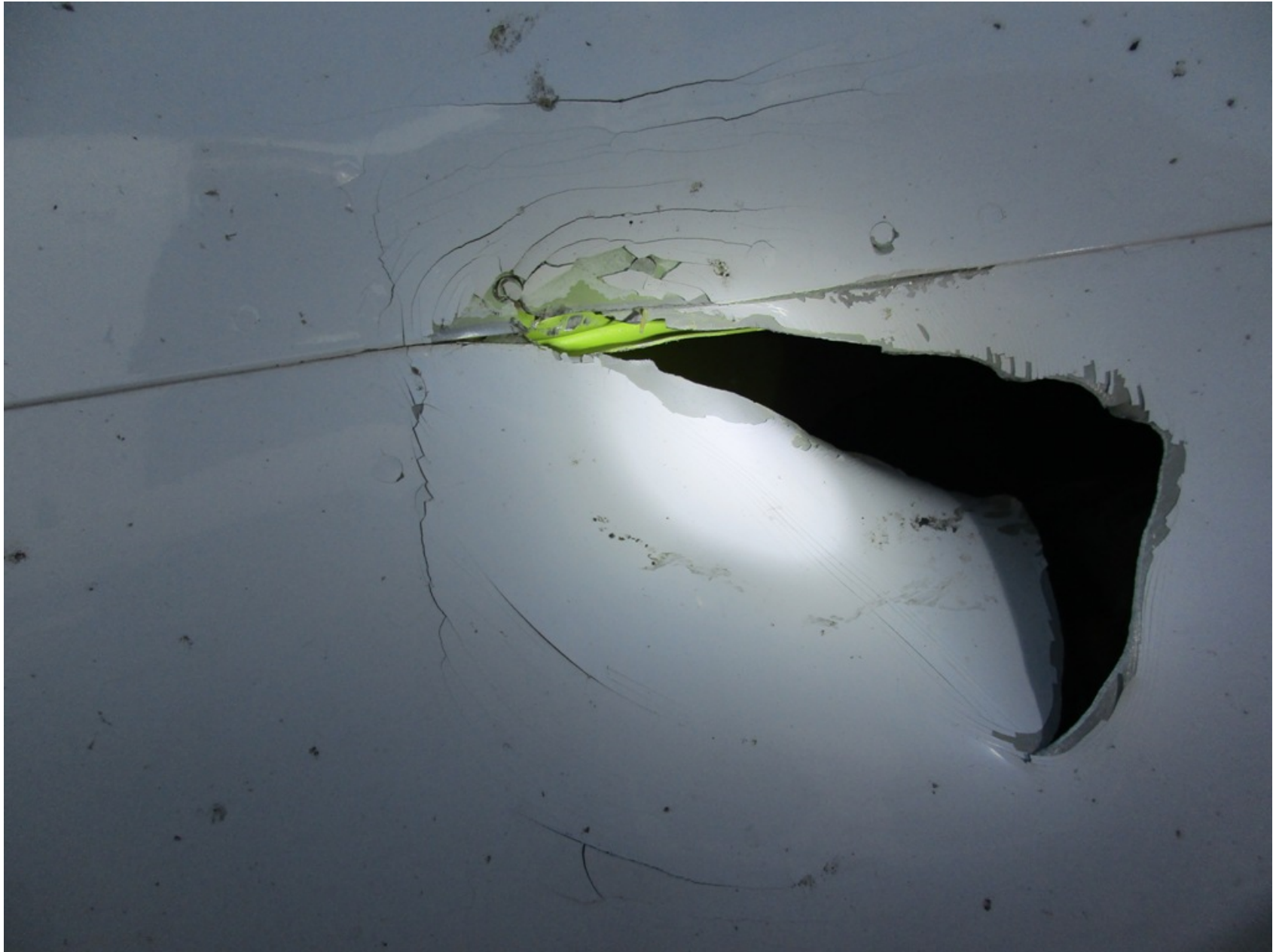
Photo 4 – Pressure Vessel Damage (FAA Photo)
