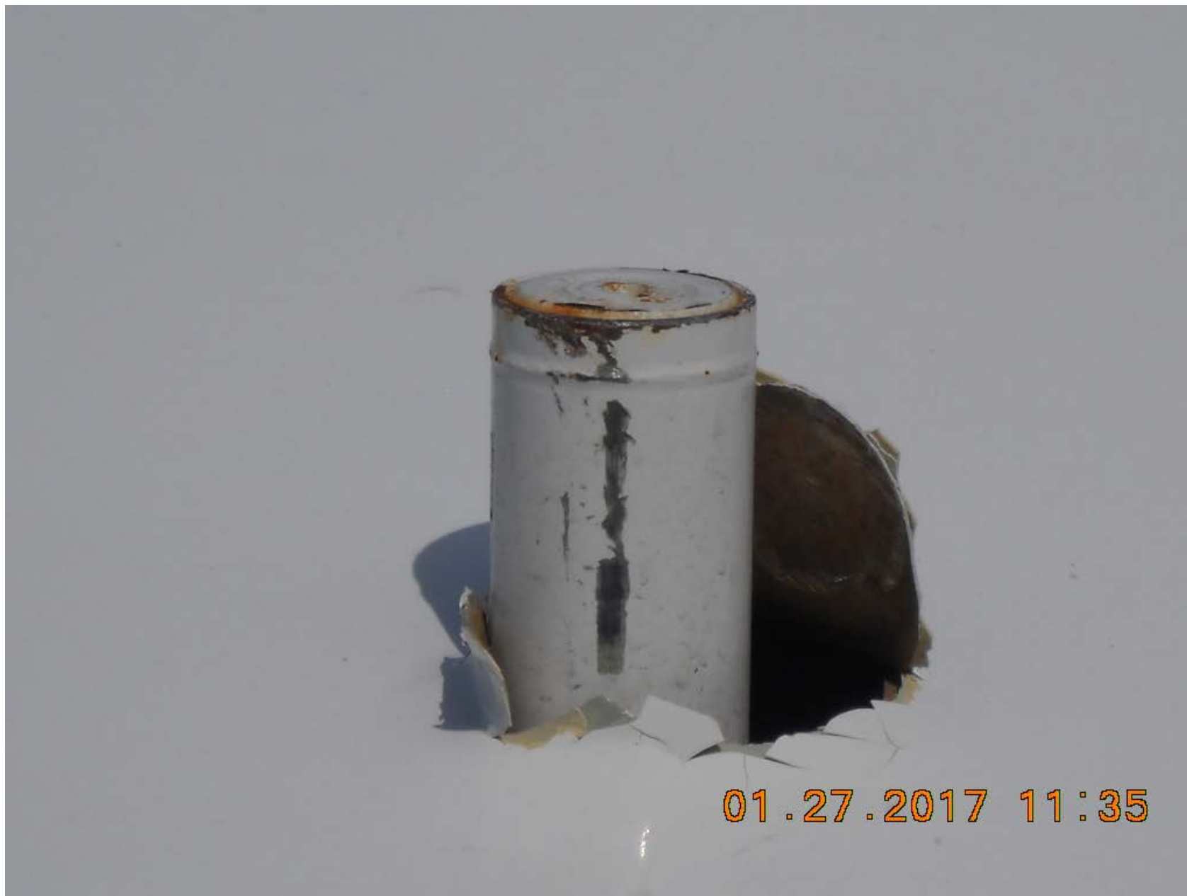
Photo 6 – Nose Gear Actuator Penetration of Upper Fuselage (FAA Photo)
