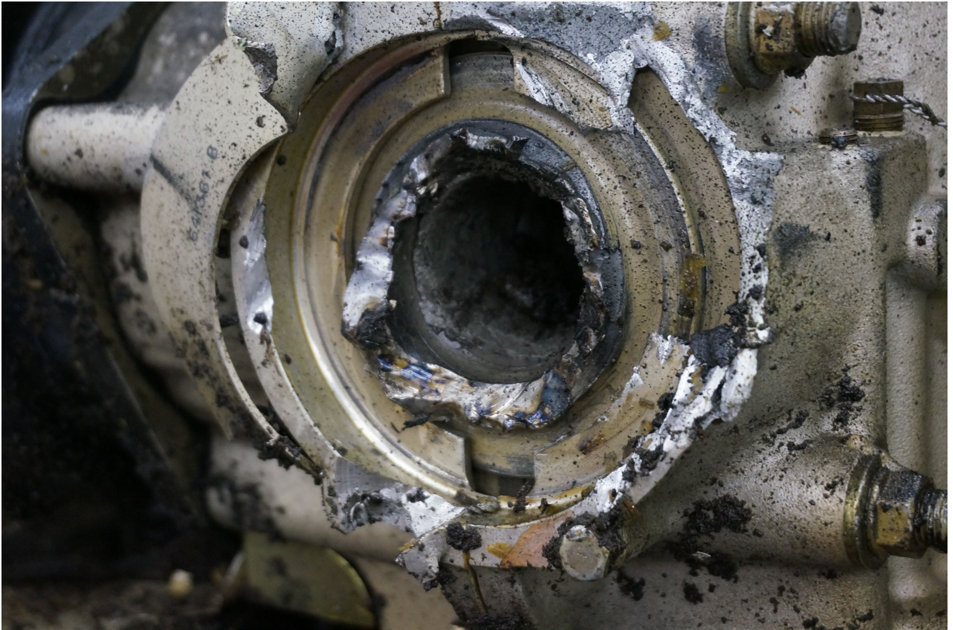
Photo 14 – Sheared End of Crankshaft in Engine
