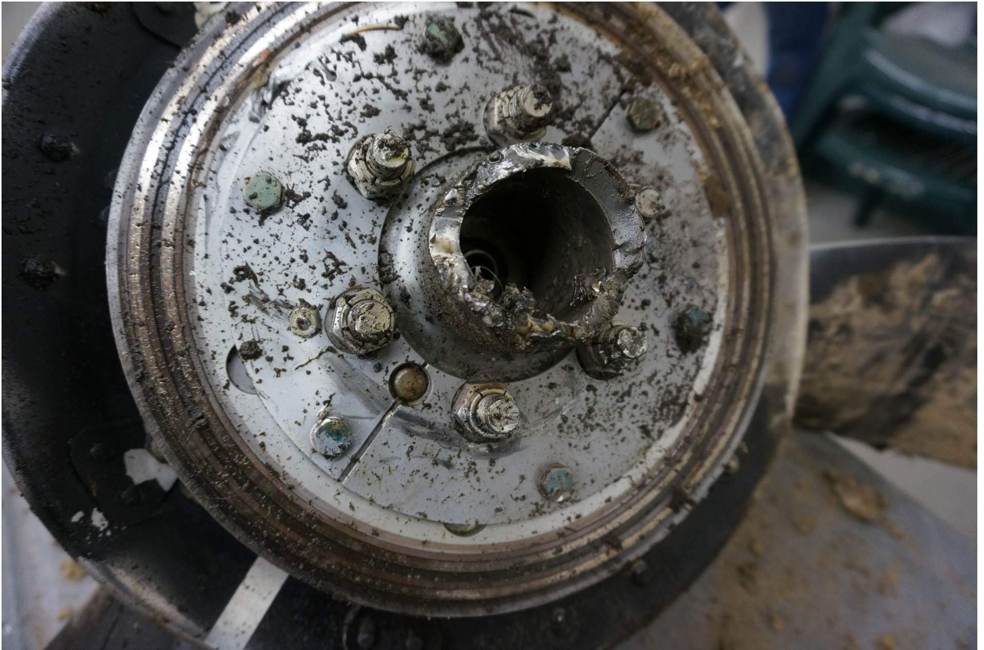
Photo 12 – Shear Face on Crankshaft End Attached to Propeller
