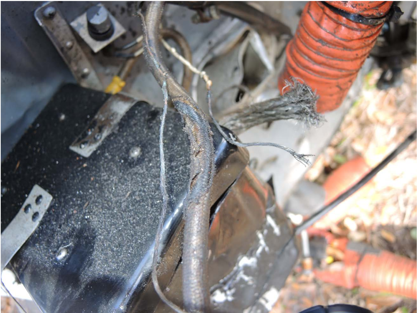
Photo 3 – View of Thermal Damage to Battery Solenoid Cable and Neighboring Wires. (Textron)
