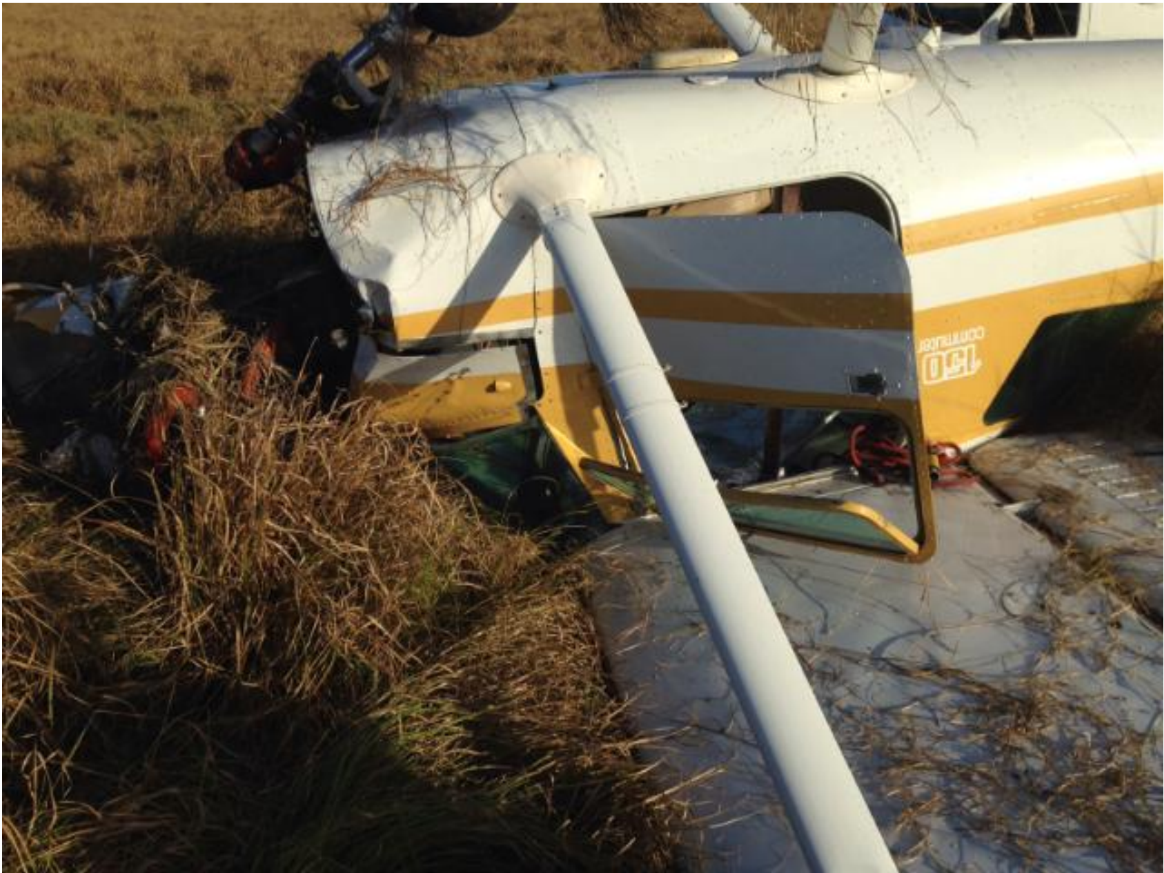
Photo 2 – View of Firewall and Fuselage Damage (F.I.T.)
