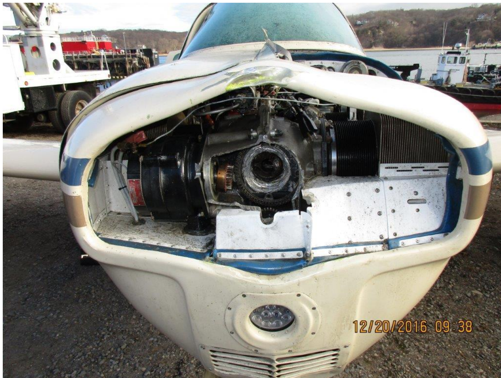
Photo 3 – Front view, missing propeller (FAA)
