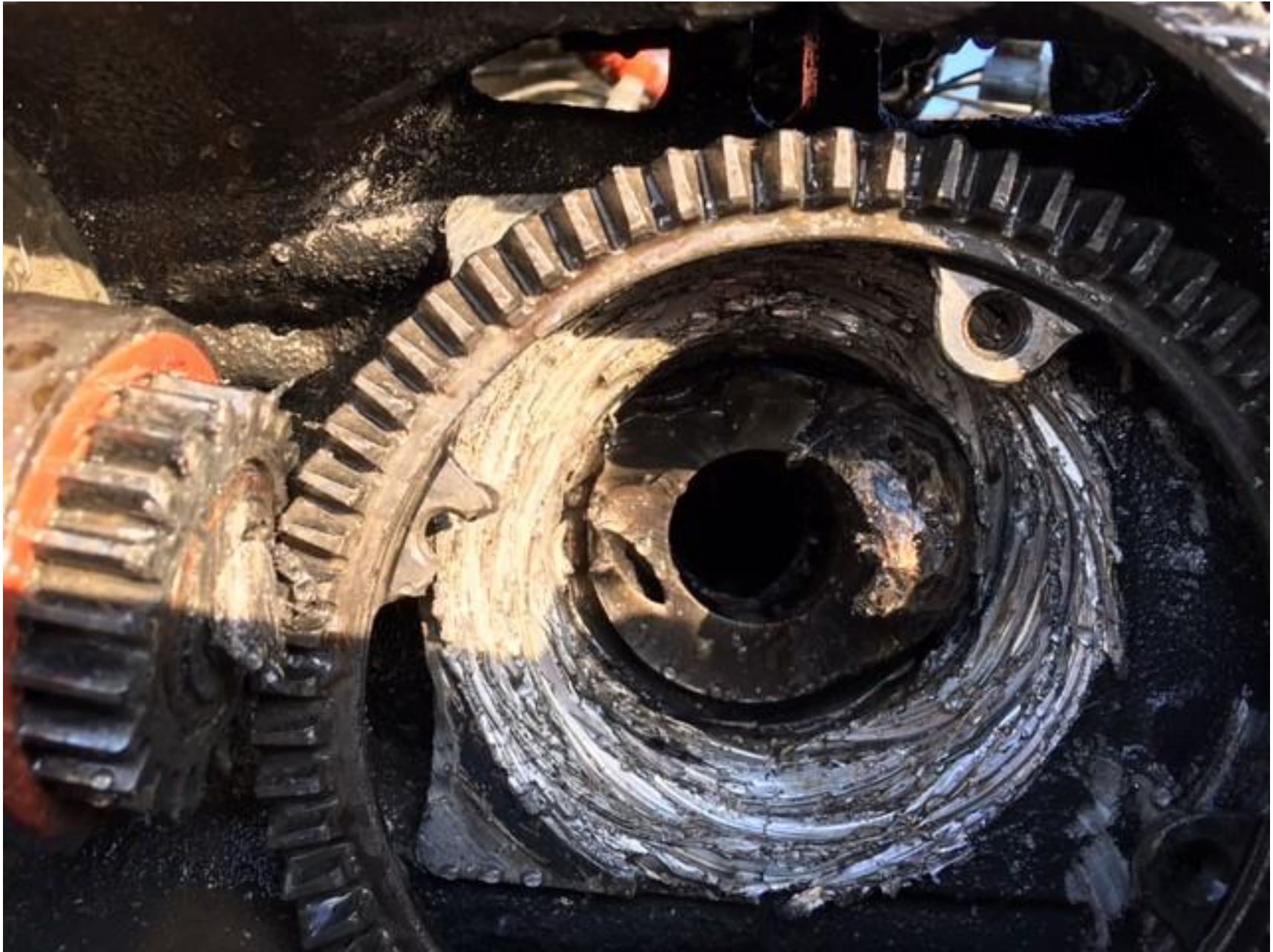
Photo 2 – Fractured Crankshaft (FAA)
