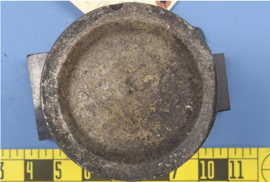
Figure 8 – View of the face of the piston crown, showing deposits, and erosion damage about the periphery.
