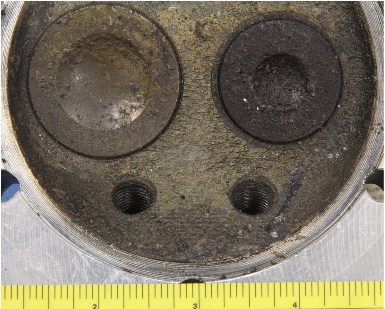
Figure 3 – A closer view of the cylinder head, showing adherent lead-based compound deposits (brownish-yellow) on the valve faces and cylinder surfaces.
