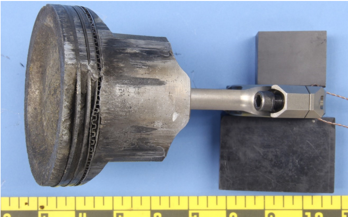
Figure 7 – Closer view of the blow-by damage on the corner of the piston crown.
