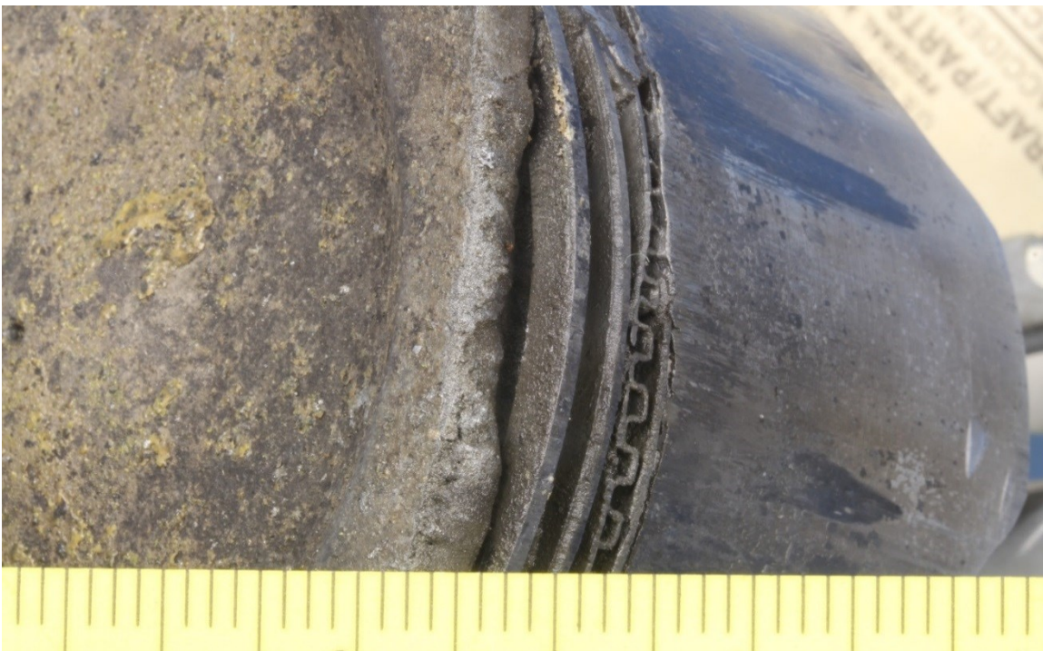
Figure 9 – View of material loss due to wear on a corner of the piston crown, showing where blowby occurred past the oil rings.
