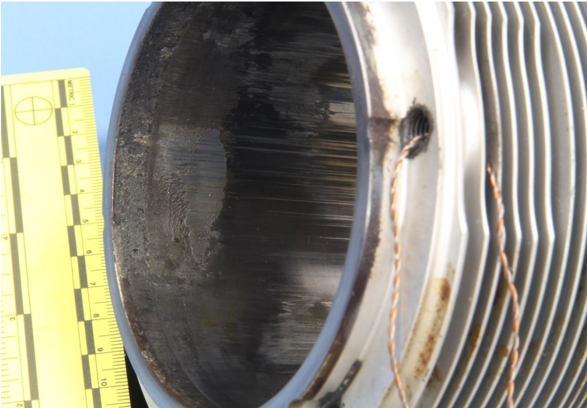
Figure 6 – Angled view of the interior of the cylinder barrel, showing sliding wear and rough erosion scars on the surface.
