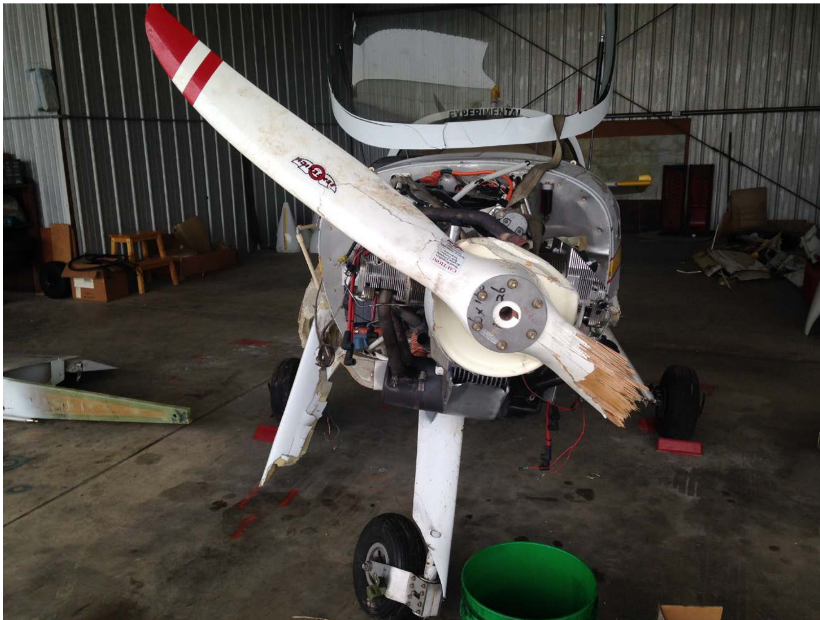
Photo 2 - Photo From Owner. Forward View of the Propeller and Engine Assembly Following Recovery. Note the Shattered propeller Blade.
