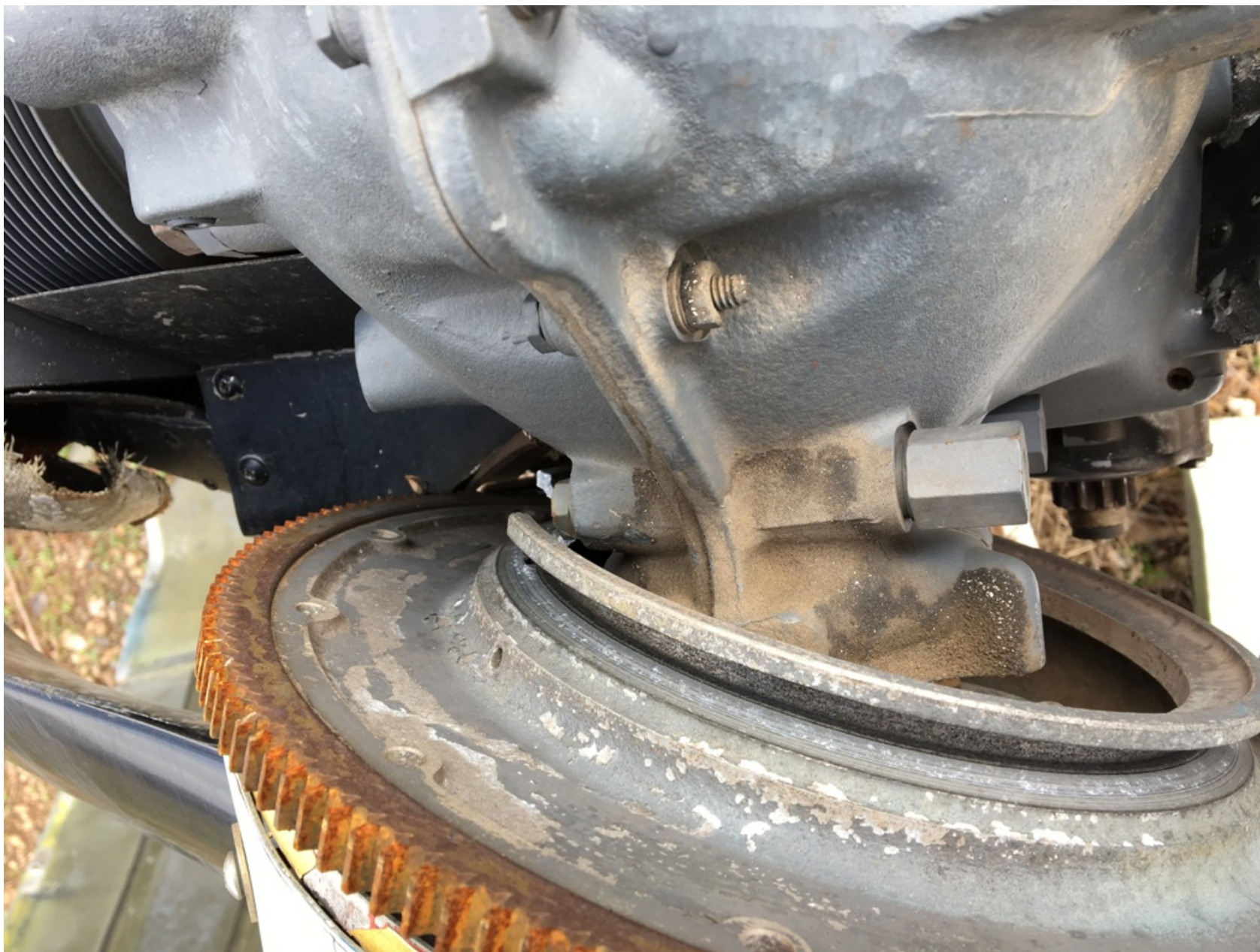
Photo 5 – Damaged Propeller Flange (NTSB Photo)
