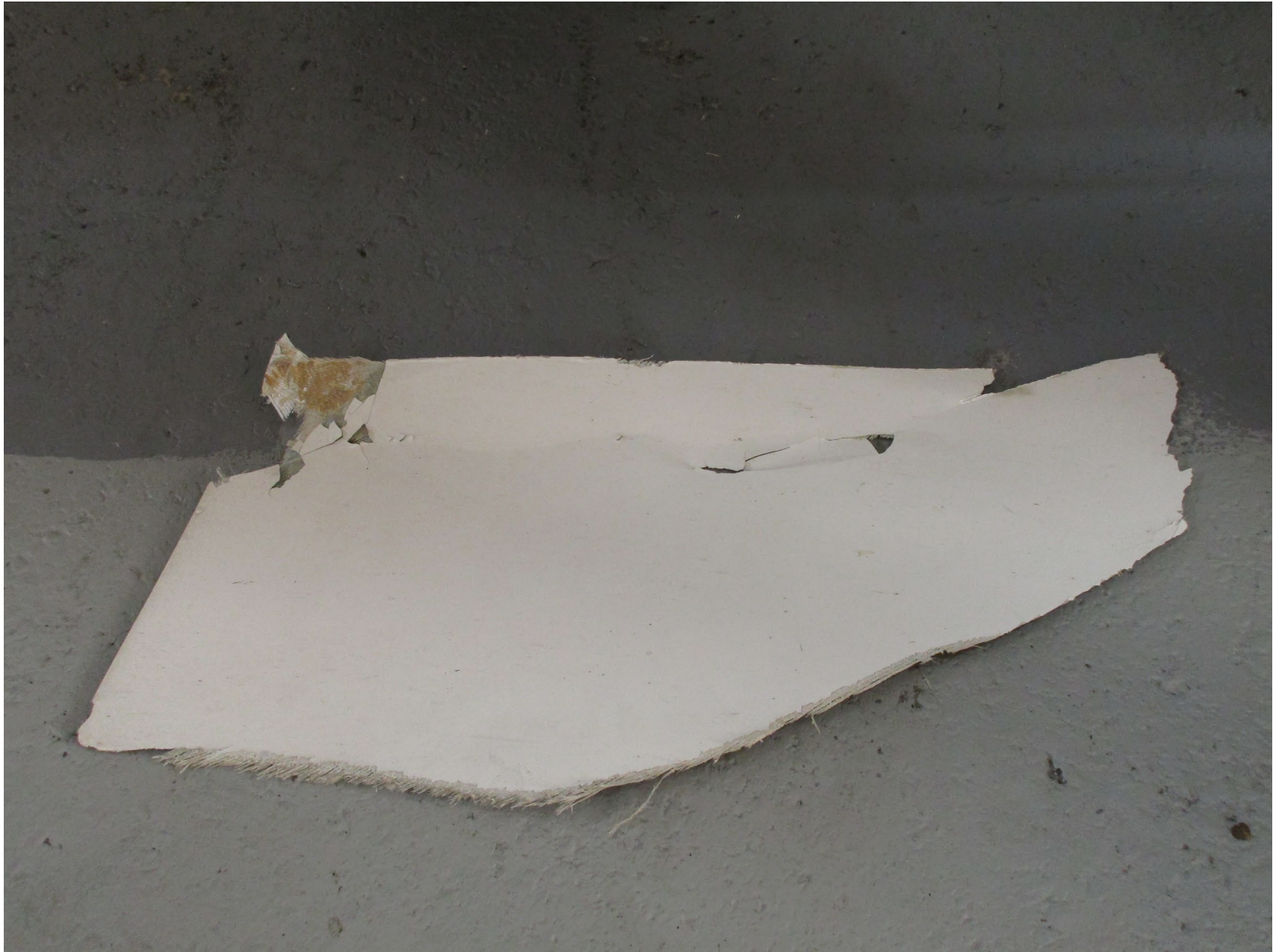
Photo 8 – Separated Section of Rudder – Courtesy of FAA
