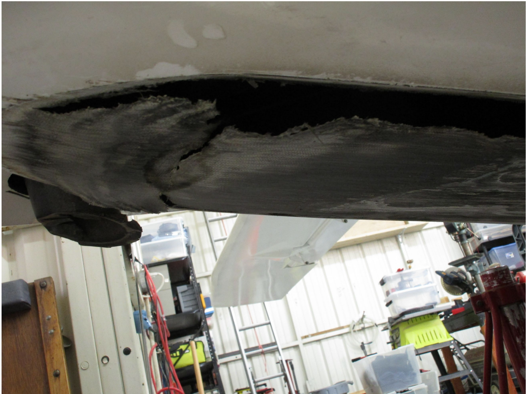
Photo 11 – Damaged Front Engine Exhaust Pipe and Lower Cowling – Courtesy of FAA
