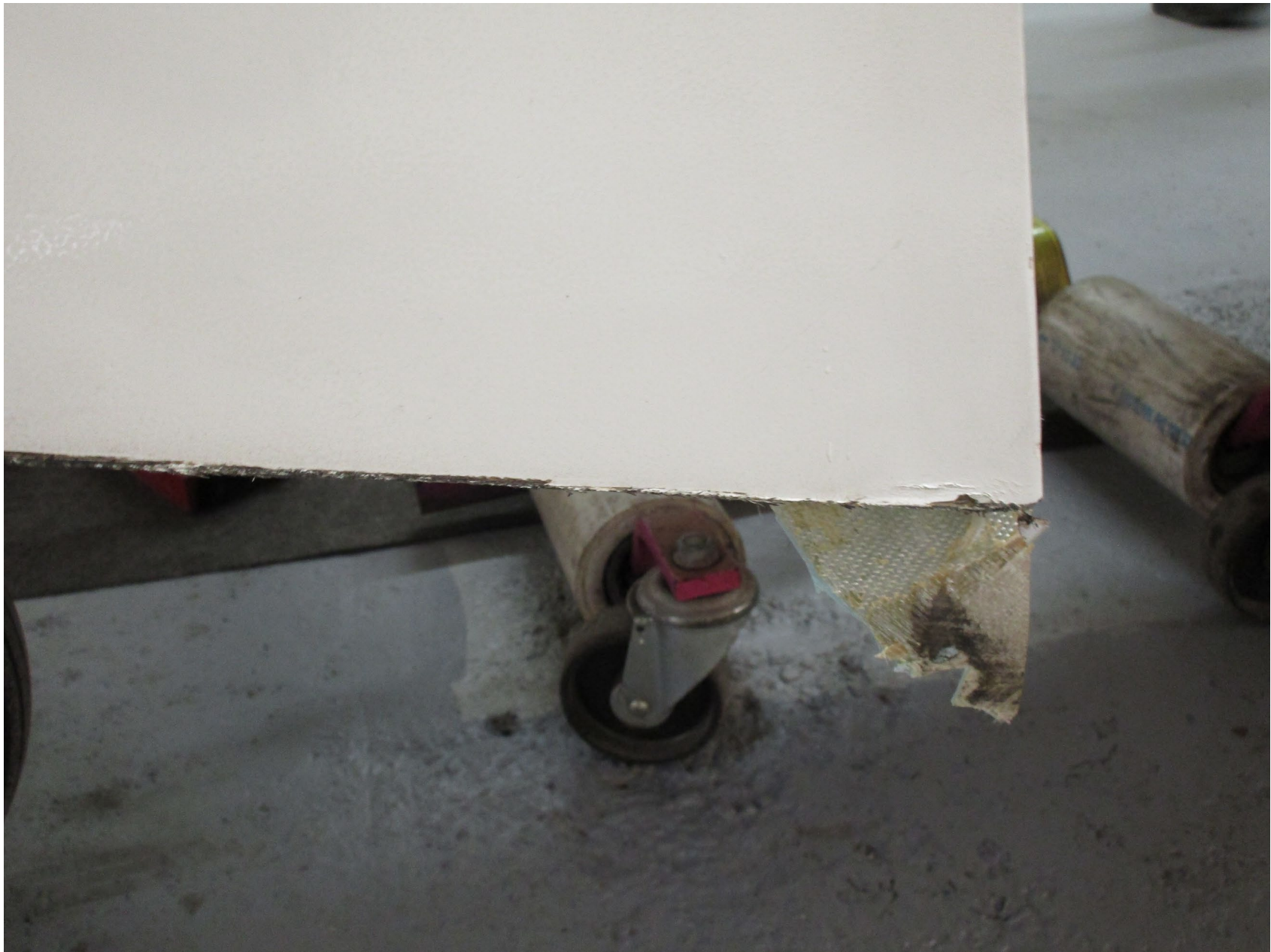
Photo 10 – Ground Down Section of Rudder – Courtesy of FAA
