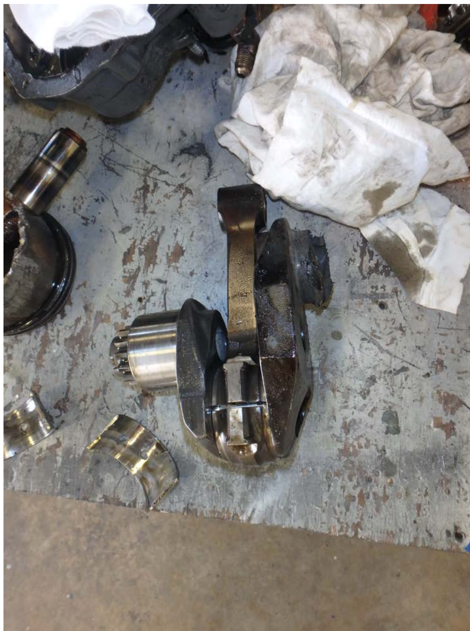
Photo 3 – View of fractured crankshaft at No. 3 bearing journal. (FAA)
