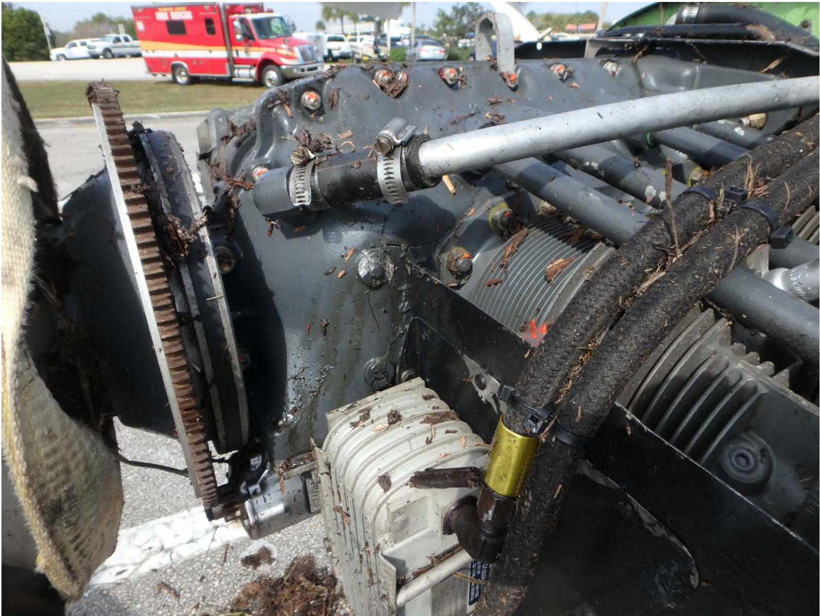
Photo 2 – View of cracked engine case after recovery. (FAA)
