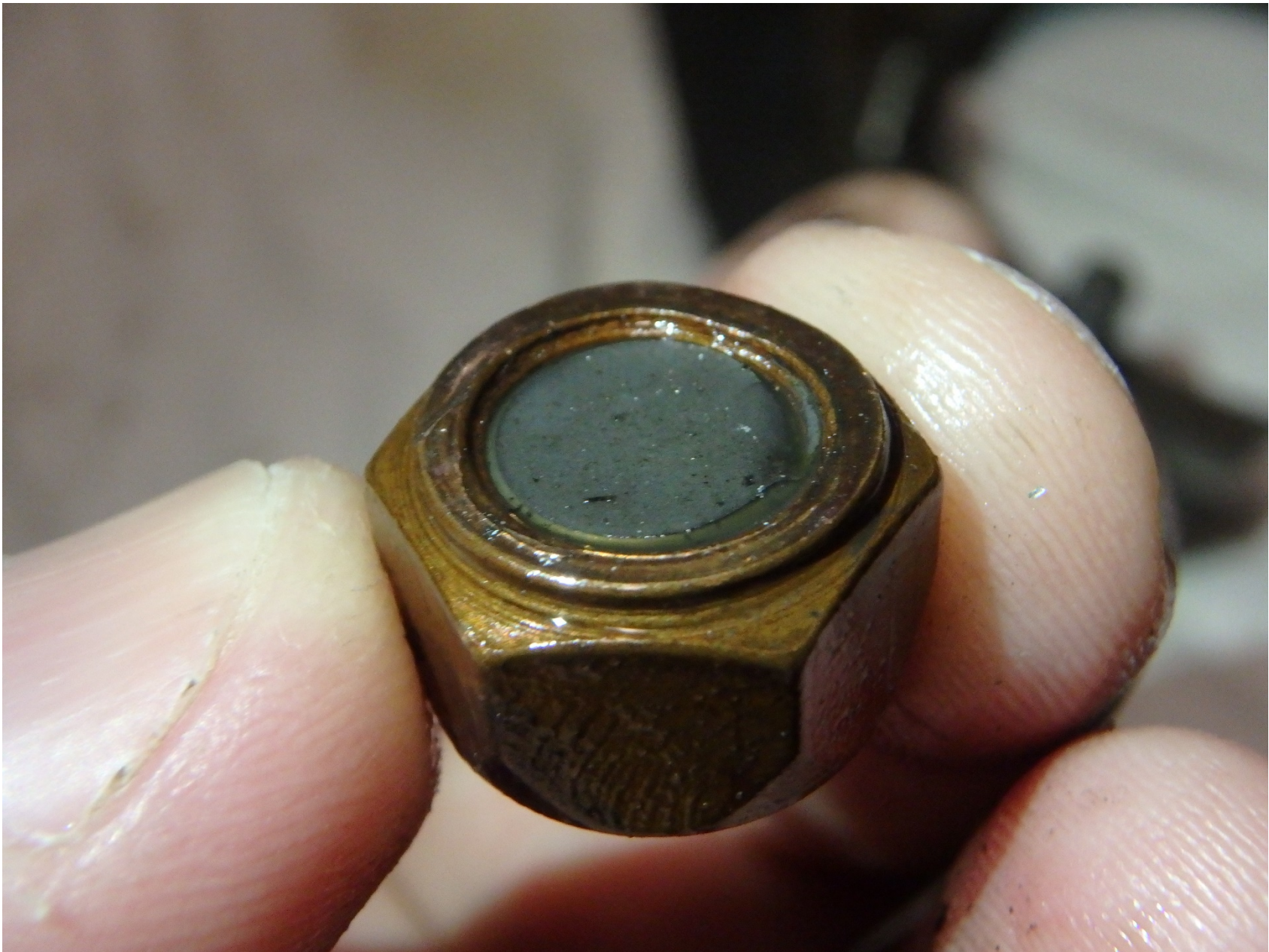
Photo 4 – View of Nut A fracture surface on raised-lip side of nut. (FAA)
