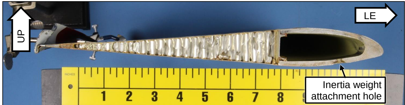
Figure 2. View of the fracture on the inboard piece of main rotor blade.
