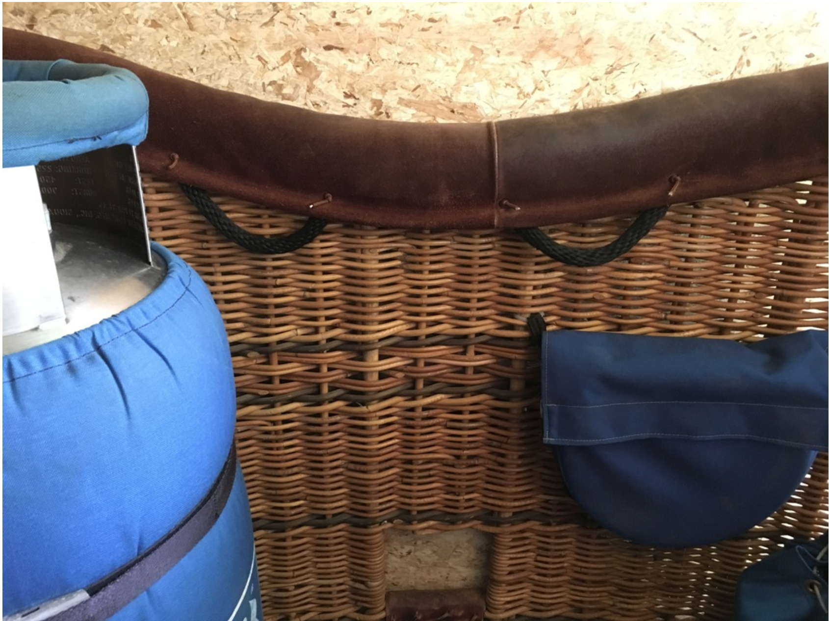
Photo 2 - Digital Photograph Provided by Pilot. Picture Depicting the Basket Handles
