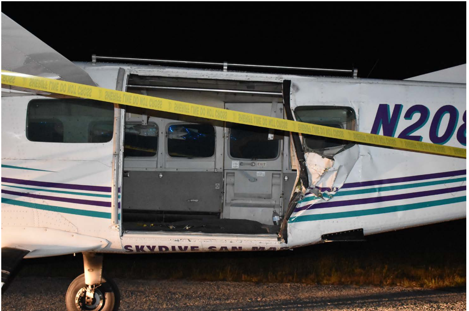
Photo 1 – Side view of cargo door showing damage to rear frame
