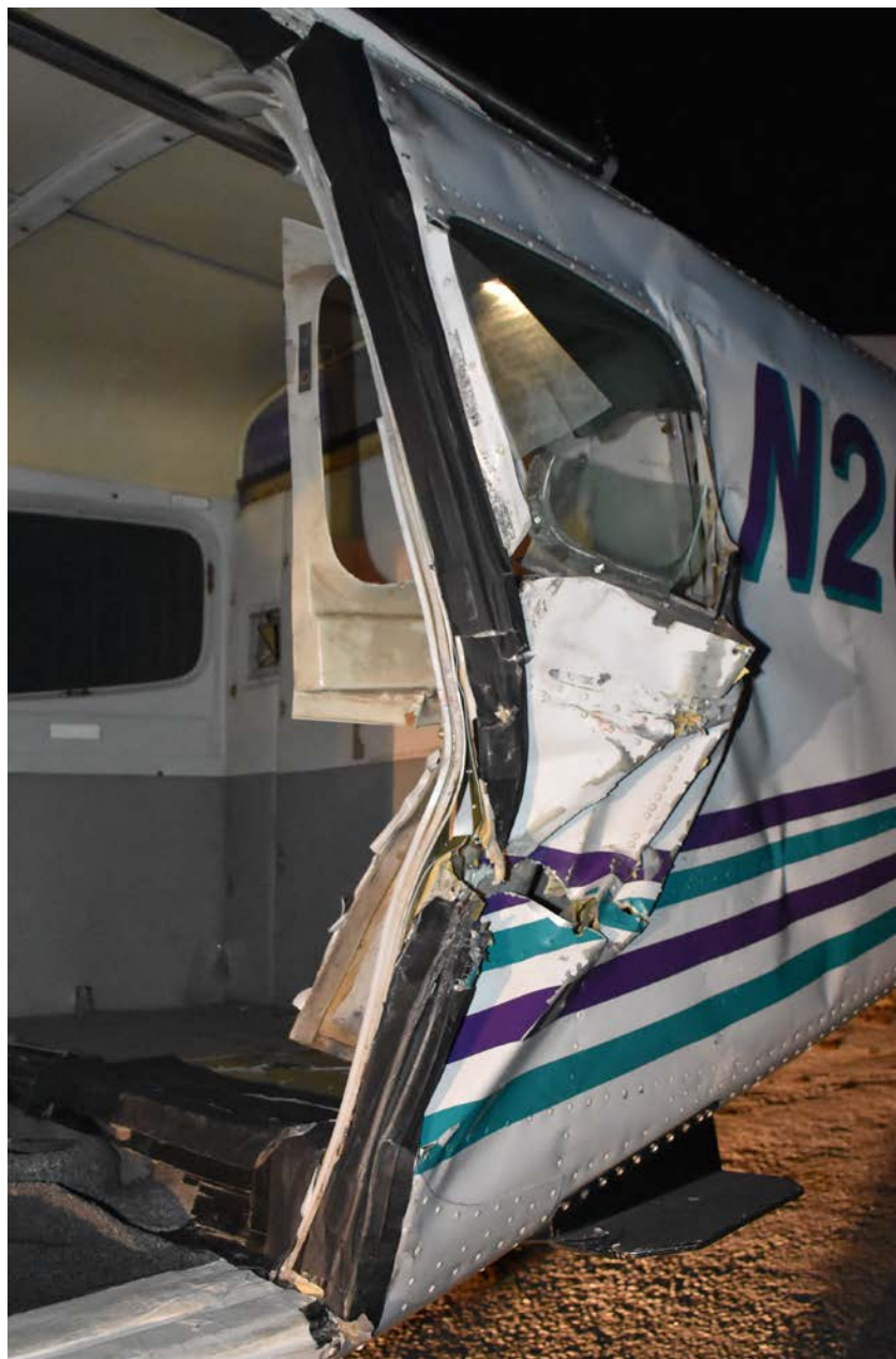
Photo 3- View of buckled fuselage and rear frame
