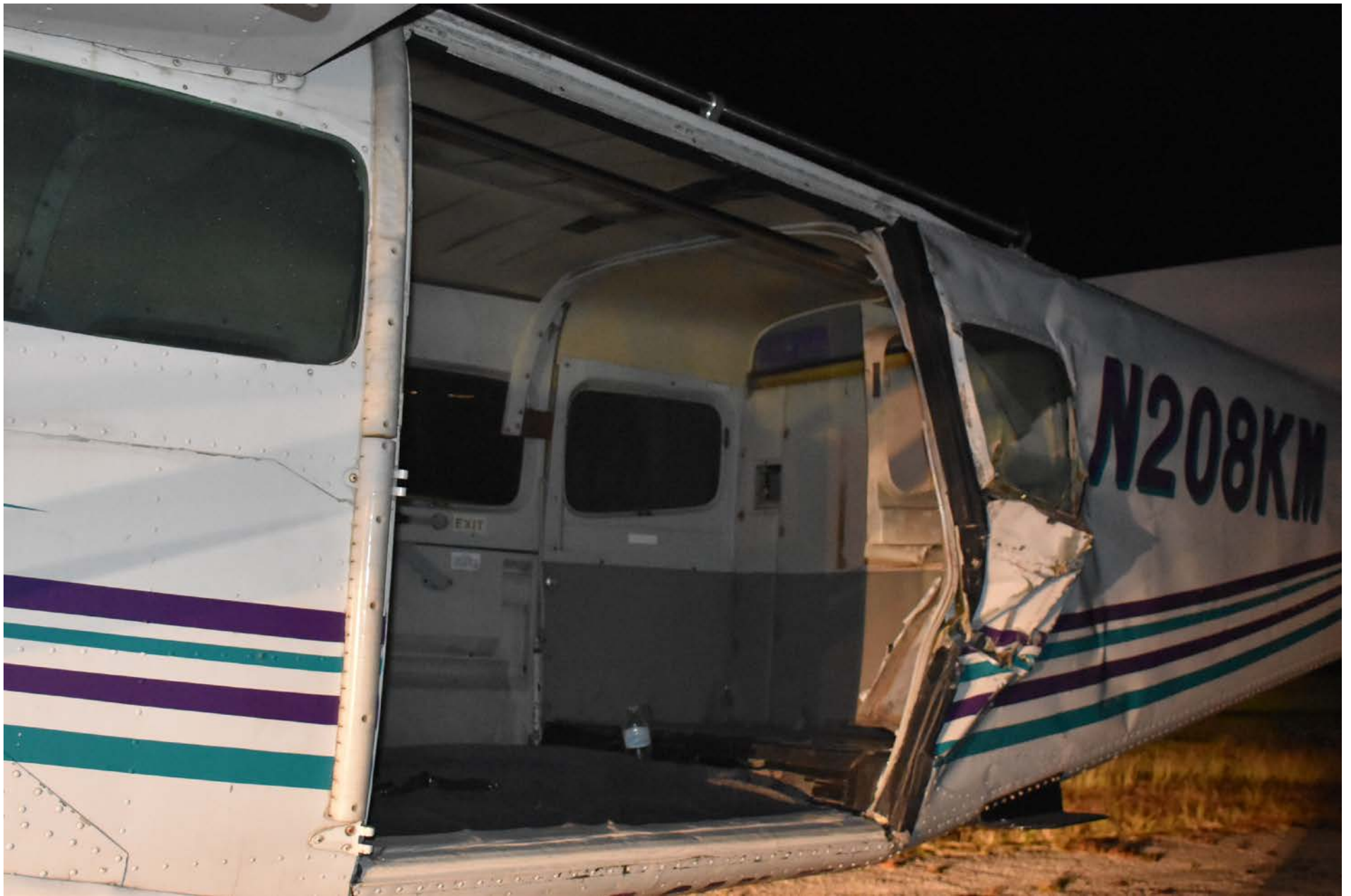
Photo 2 - Forward view of cargo door showing damage to rear frame
