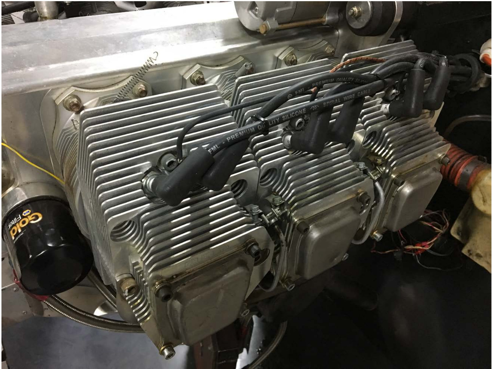
Photo 4 – Engine, Numbers 2, 4, and 6 Cylinders
