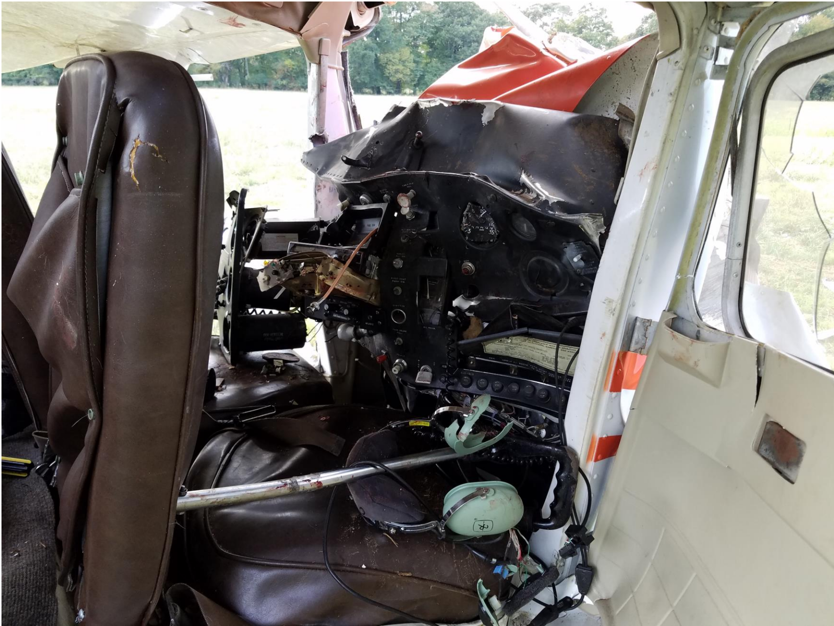
Photo 5 – Cockpit interior damage. (Courtesy of FAA)
