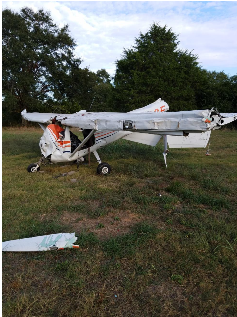
Photo 2 – Left side of airplane damage. Note flattened out engine compartment and leading edge damage to both wings. (Courtesy of FAA)
