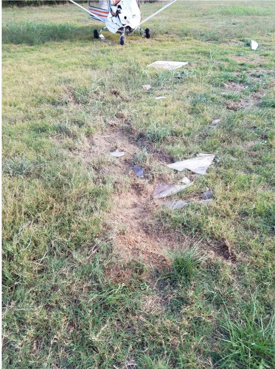
Photo 3 – Photograph of impact ground scars. (Courtesy of FAA)
