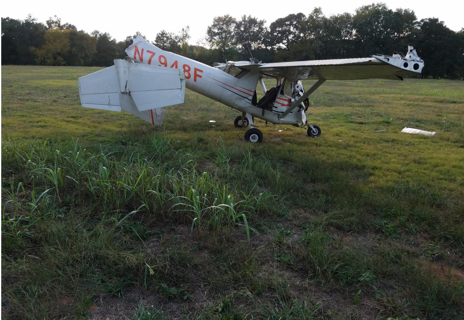
Photo 1 – Right side of airplane damage and severed tail. (Courtesy of FAA)
