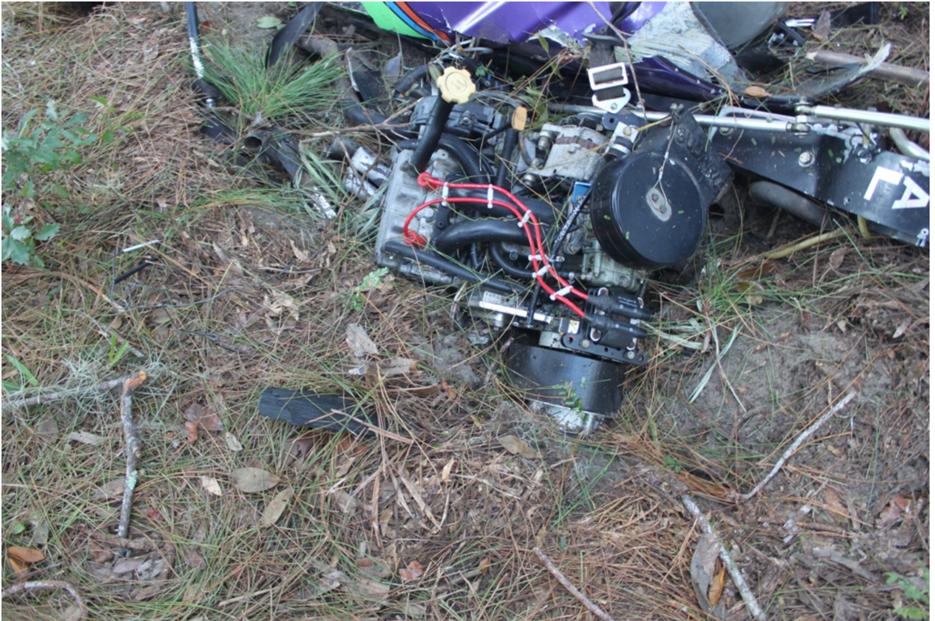
Photo 2 - NTSB Digital Photograph. View of the Engine Assembly at the Accident Site. Note the Ignition Control Module.
