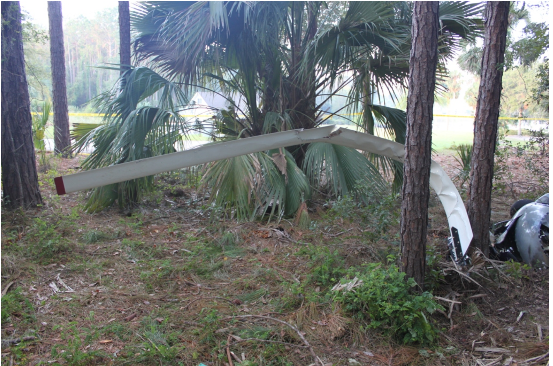
Photo 4 - NTSB Digital Photograph. View of the Damage to One of the Main Rotor Blades.
