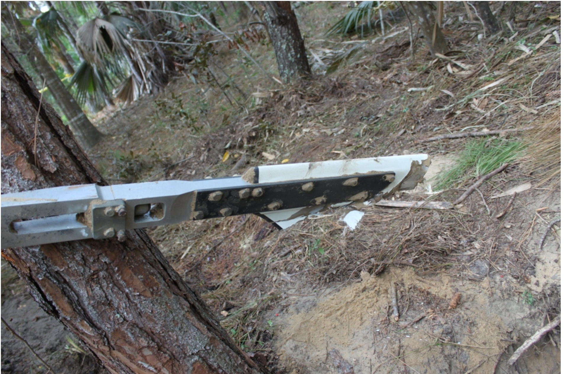
Photo 6 - NTSB Digital Photograph. View of the Remaining Section of the Fractured Main Rotor Blade that Was Buried in the Ground.
