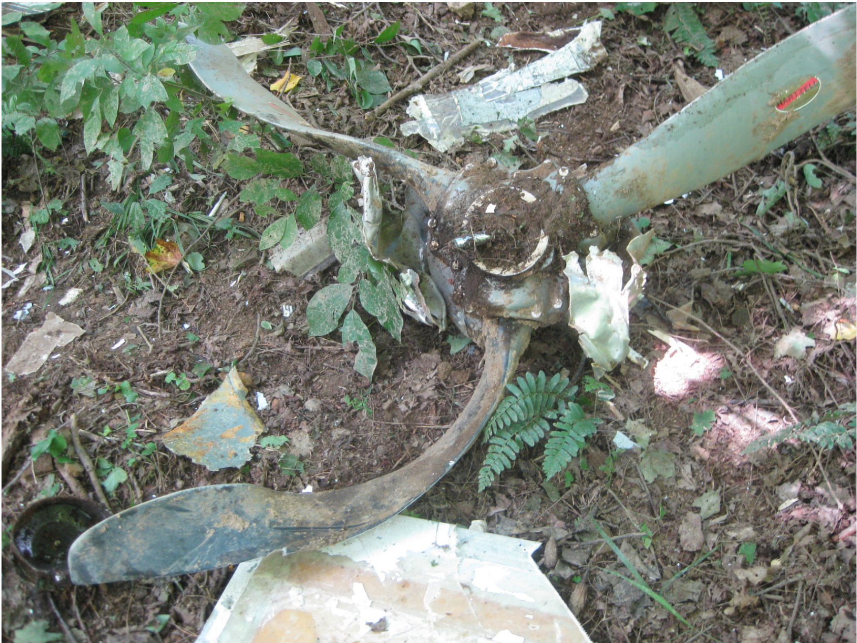
Photo 5 – View of damaged propeller separated from engine
