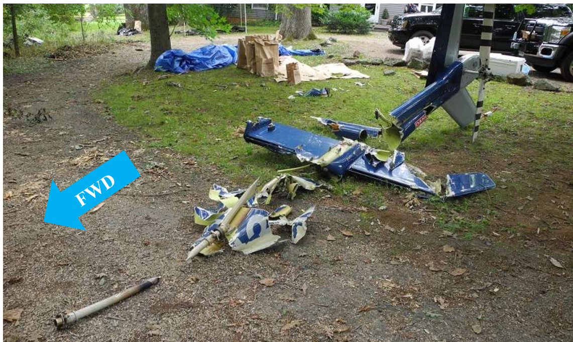
Figure 4. A reconstruction of the recovered tail rotor drive train.
