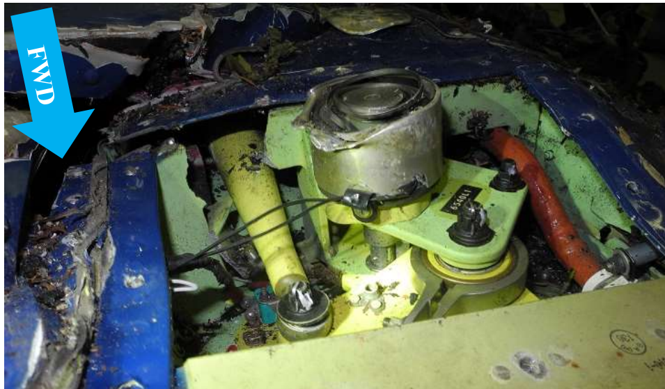
Figure 6. The pedal bell crank and PRCS solenoid.
