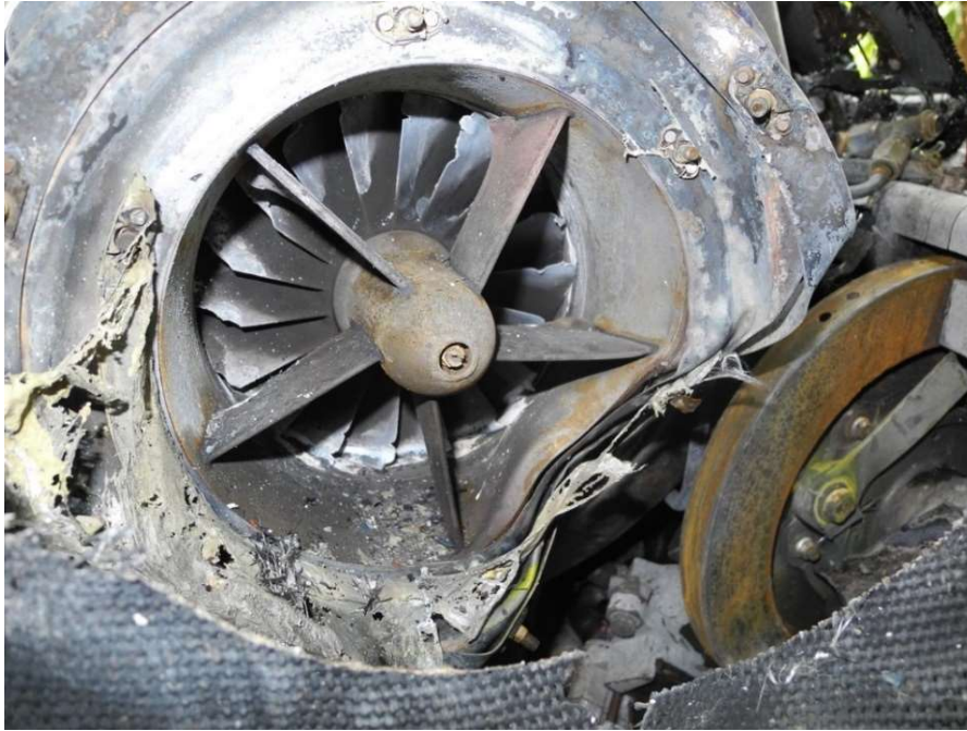
Figure 8. The engine inlet vanes and the first stage compressor blades.
