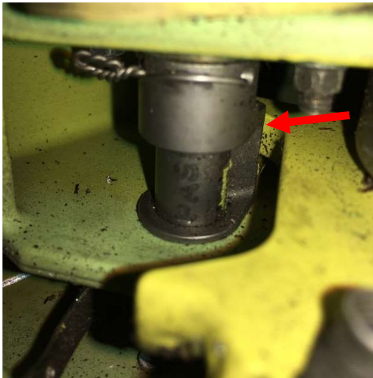
Figure 7. The PRCS cam (red arrow) found in the engaged position.
