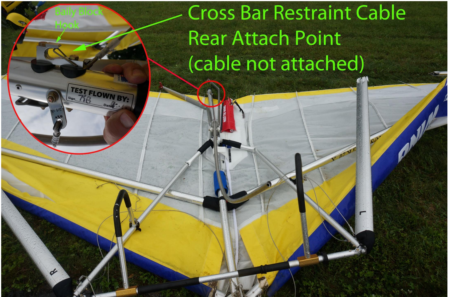
Cross Bar Restraint Cable – Rear Attach Point
