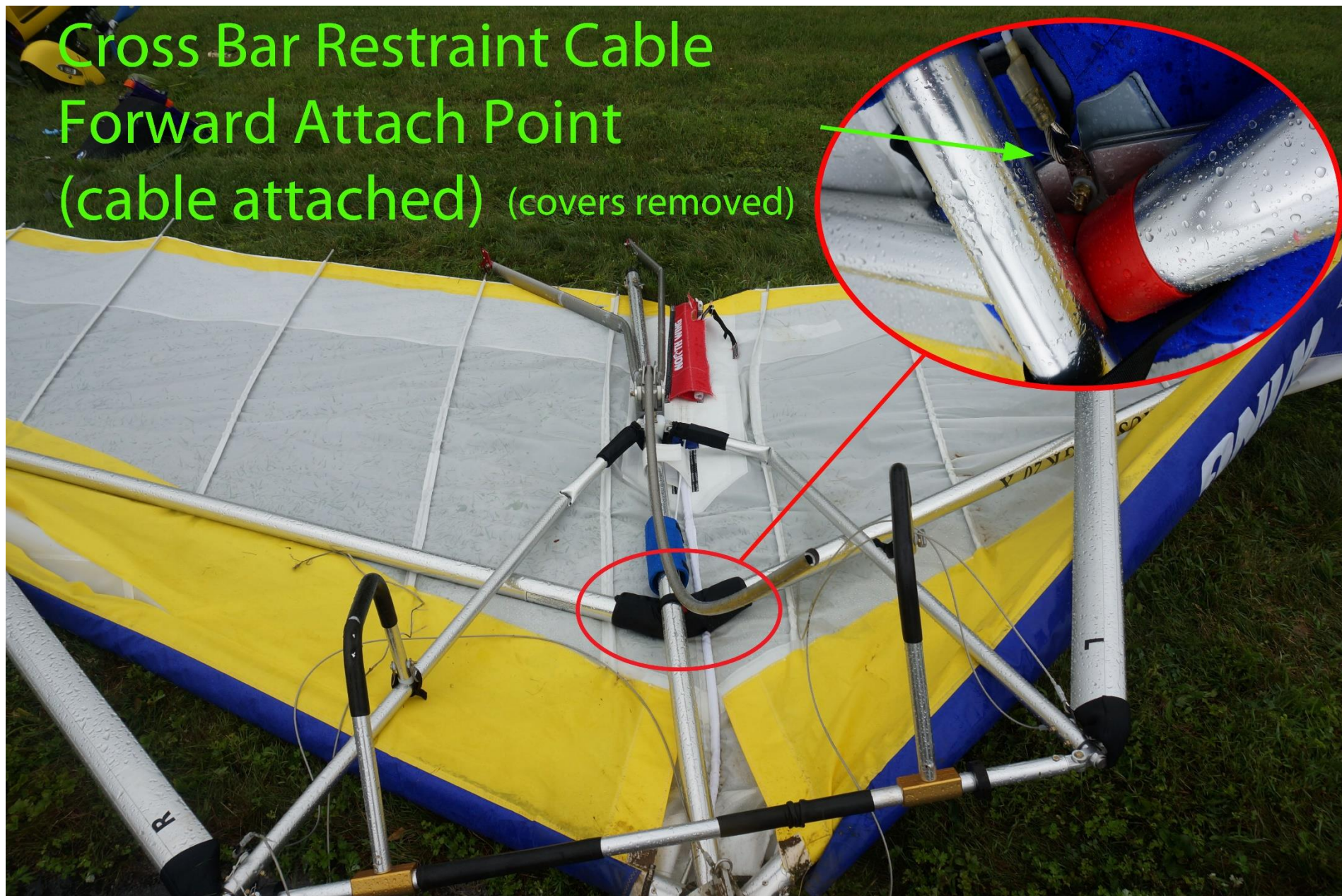
Cross Bar Restraint Cable – Forward Attach Point
