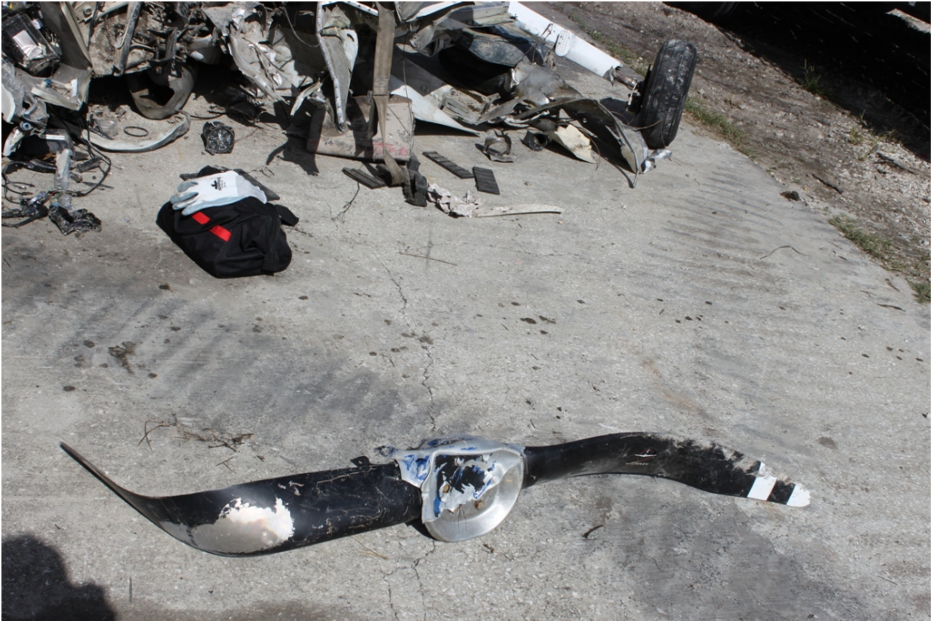
Photo 11 - NTSB Photograph Depicting the Propeller. Note the Blade Bending and Damage.
