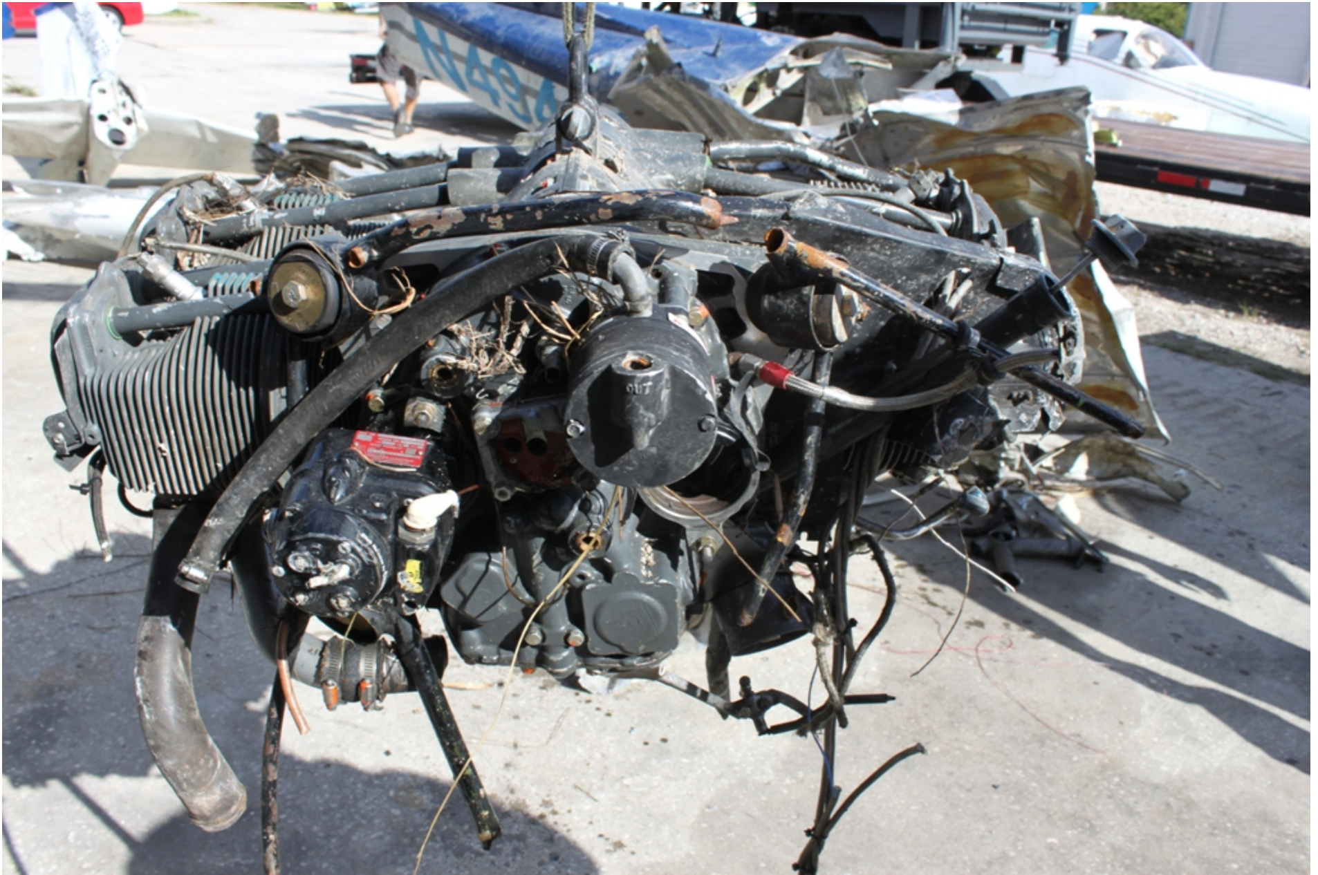
Photo 9 - NTSB Photograph Depicting the Rear Side of the Engine Assembly, and View of the attached Engine-Driven Vacuum Pump.
