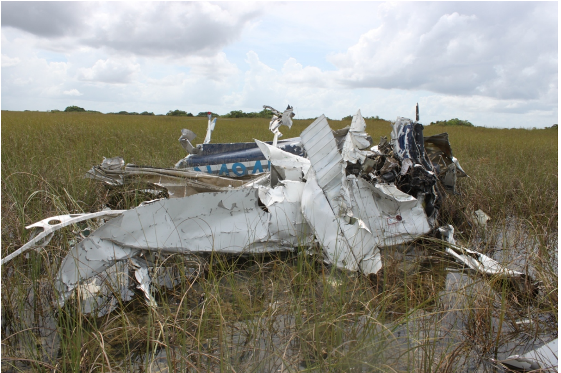
Photo 5 - NTSB Photograph Depicting Closer View of the Wreckage at the Accident Site. Note the extensive damage to the Right Wing, Cockpit, and Fuselage.
