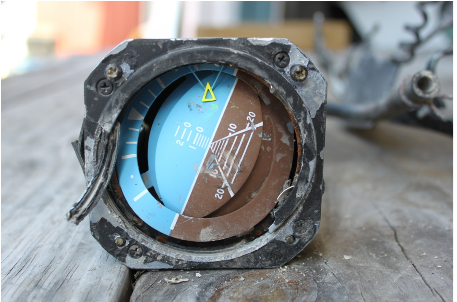
Photo 13 - NTSB Photograph Depicting the Attitude Indicator Following Removal from Behind The Instrument Panel. Note the Fixed Pointer Position.
