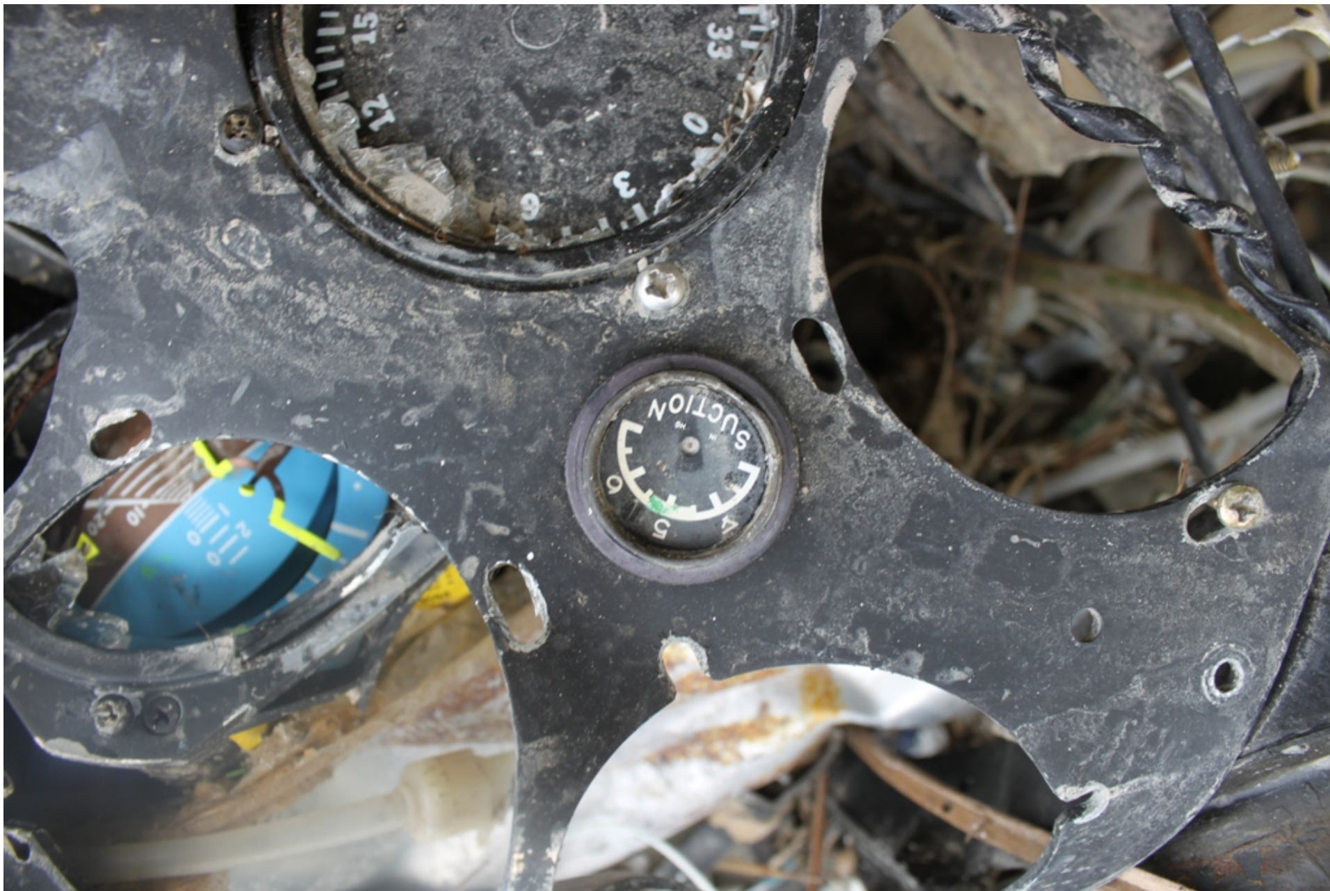
Photo 6 - NTSB Photograph Depicting a Section of the Instrument Panel Containing the Suction Gauge, Separated Attitude Indicator, and Portion of Directional Gyro.
