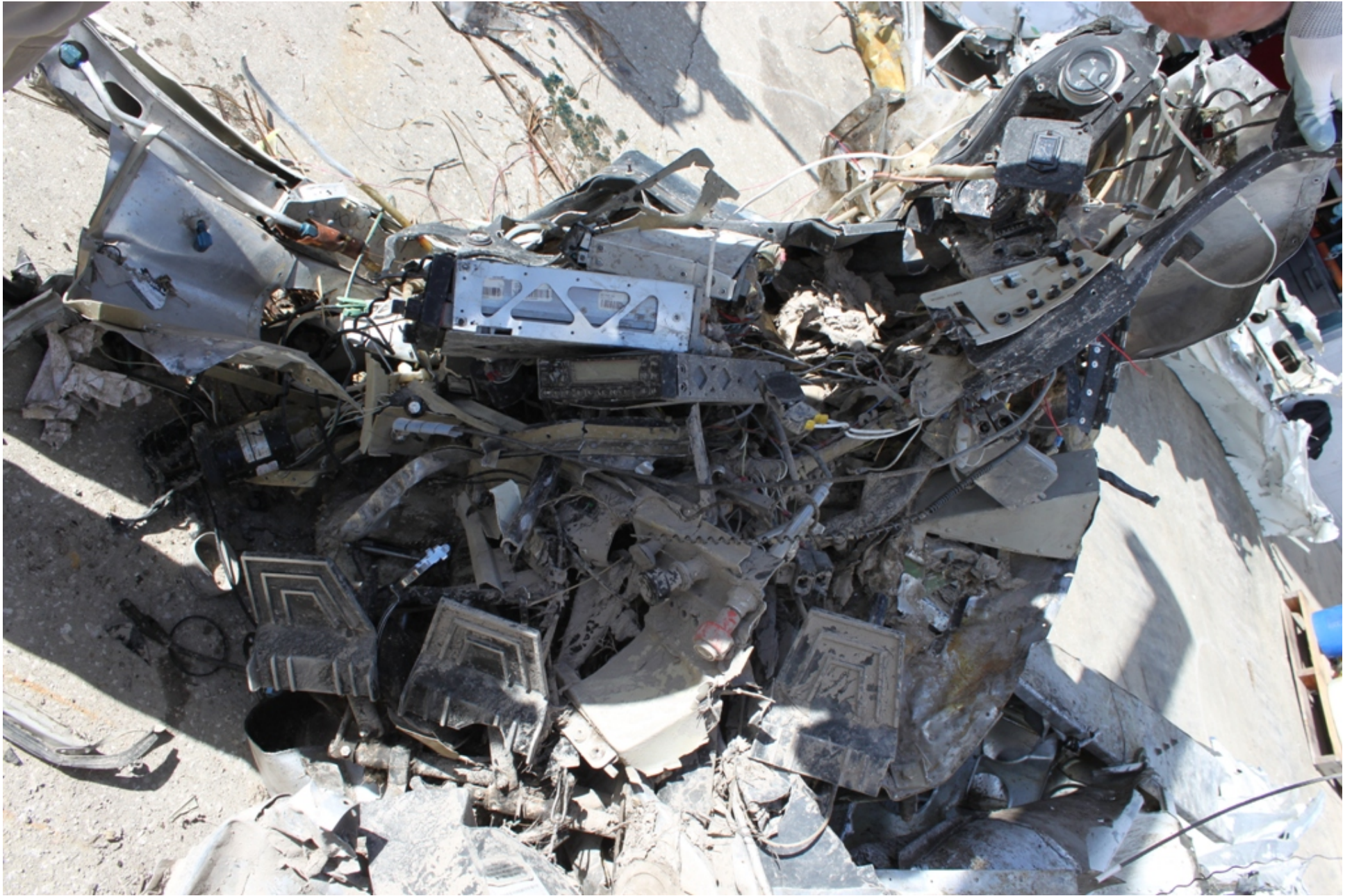
Photo 10 - NTSB Photograph Depicting the Instrument Panel, Throttle Quadrant, Rudder Pedals, Avionics, and Instruments.
