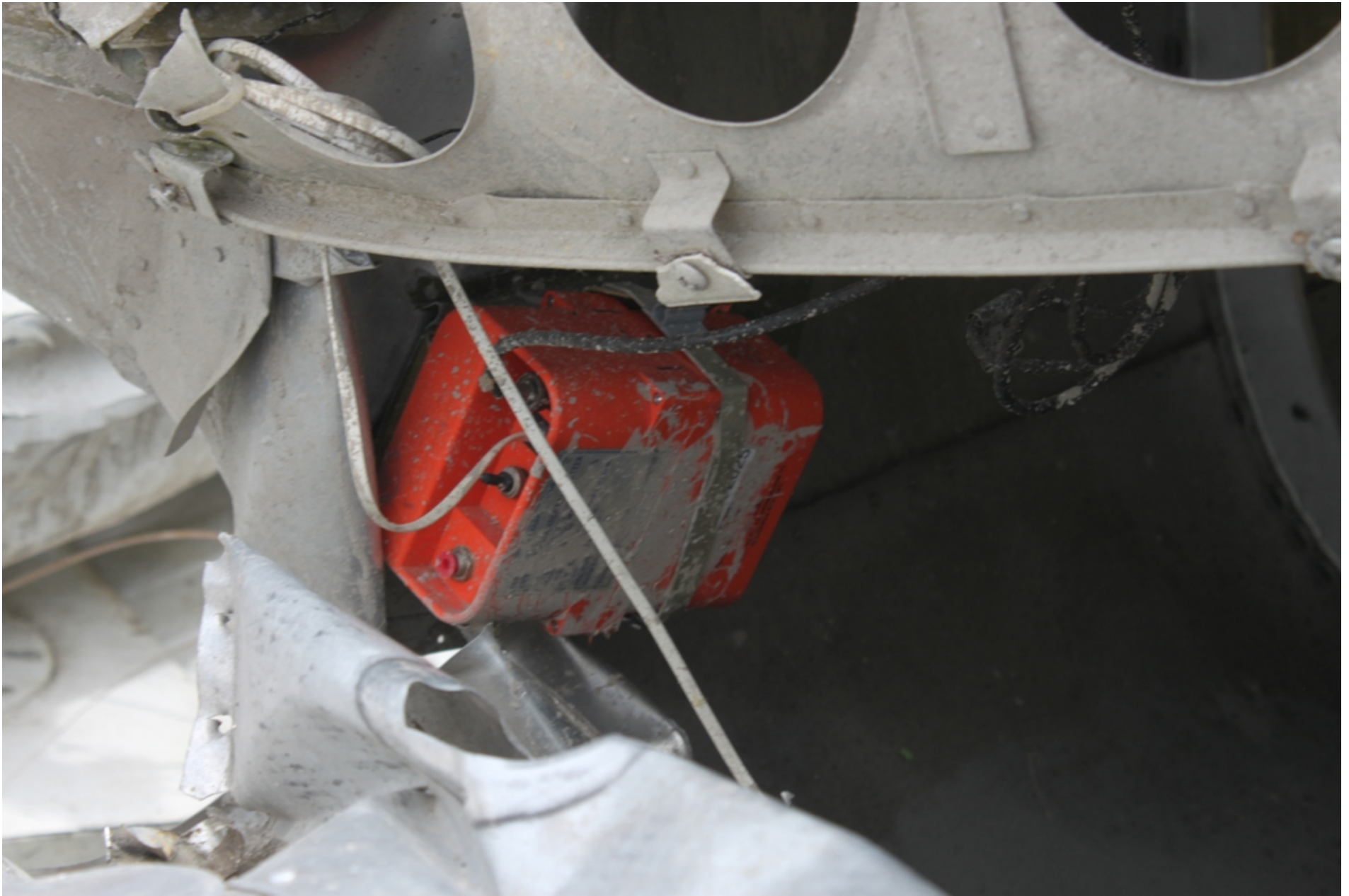
Photo 7 - NTSB Photograph Depicting the Emergency Locator Transmitter (ELT) as First Viewed. Note the ELT is Partially Out of Its Bracket.
