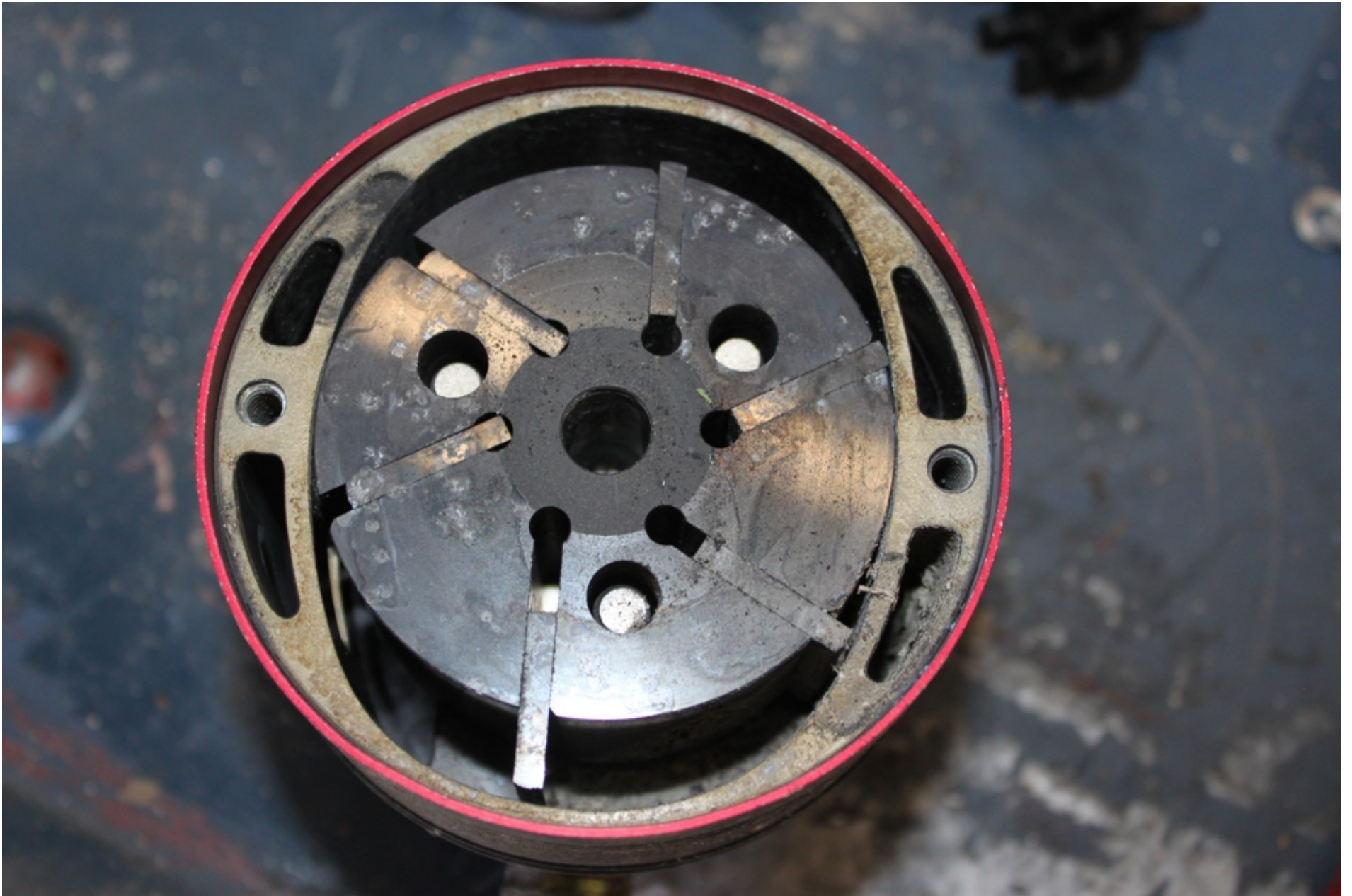
Photo 14 – NTSB Photograph of the Engine-Driven Vacuum Pump Showing the Intact Rotor and Vanes.
