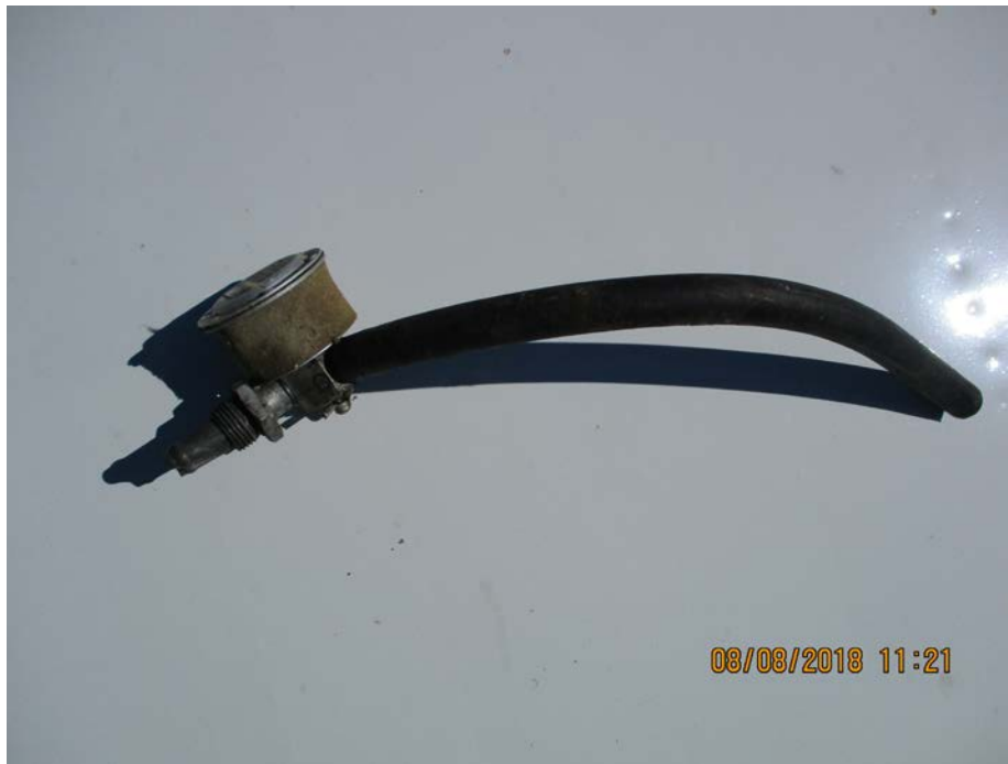
Photo 5. Regulating valve with a 12 inch long hose attached.
